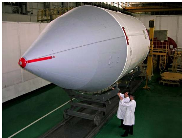
FIG. 6. Payload fairing from Lavoshkin Association
