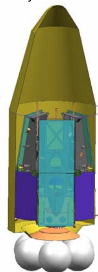
Figure 2 The three SAR satellites can all be accommodated in a Soyuz for a joint launch
