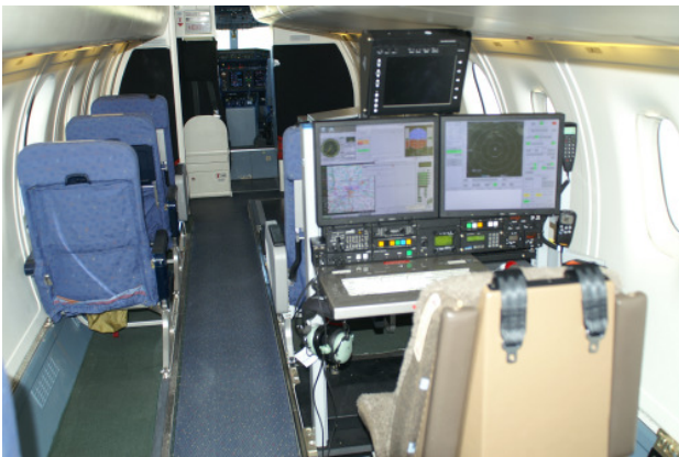
FIG. 15: Cabin view of the installed AeroMission work station
