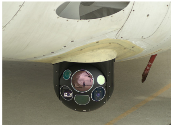
FIG. 4: The turret of the electro-optical/infrared sensor
