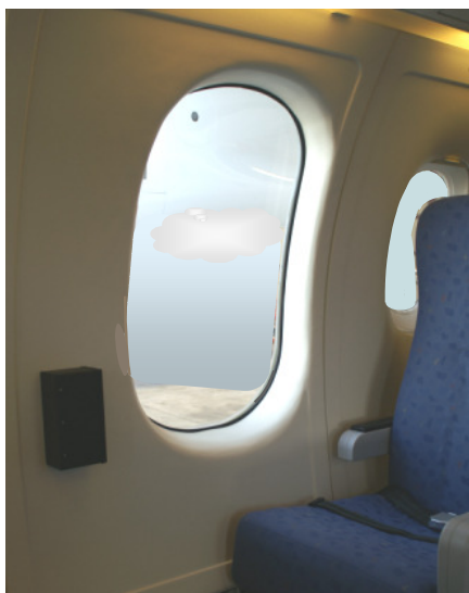
FIG. 16: The enlarged observation windows (DO 328)
