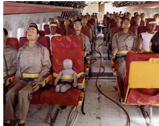
NASA Dryden Flight Research Center Photo Collection http://www.dfrc.nasa.gov/gallery/photo/index.html NASA Photo: ECN-26307 Date: 1984 Controlled Impact Demonstration instrumented test dummies installed in plane
