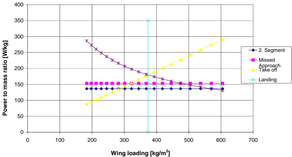
Figure 9: Matching chart for the sizing process of the ATR 72.
