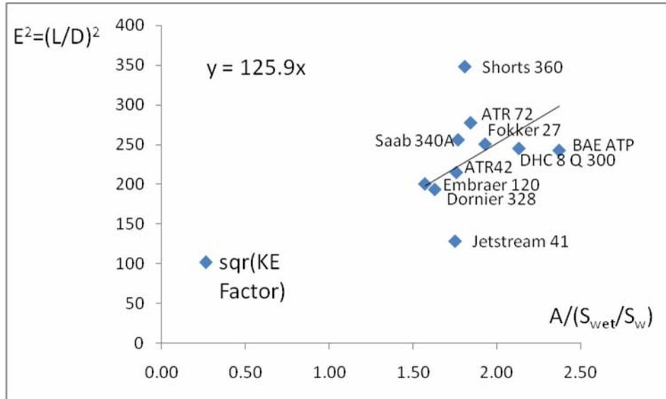
Figure 8: Statistical factor  $k_E$  for calculating the maximum glide ratio  $E_{max}$ , for turboprop aircraft based on data from [11].
