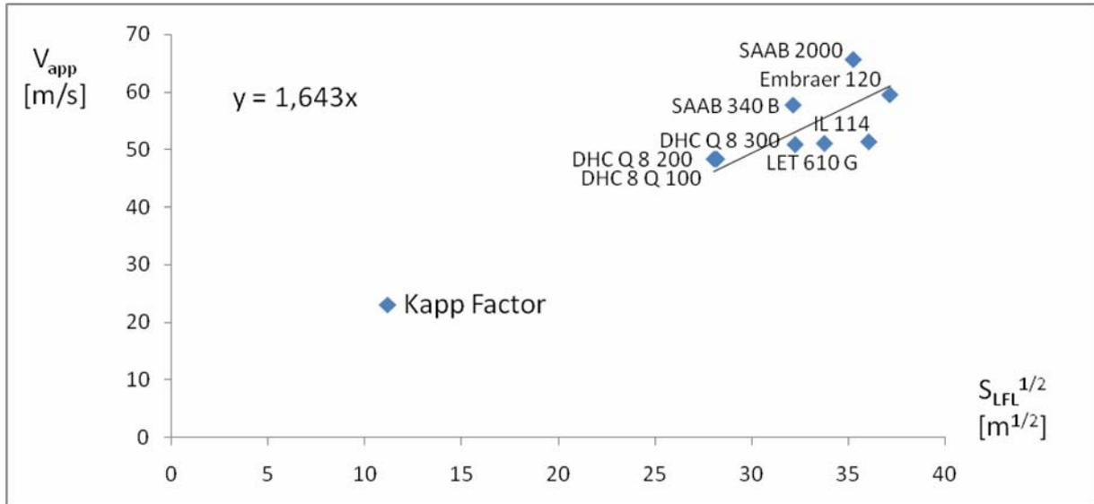
Figure 4: Statistical factor  $k_{APP}$  for approach speed calculation from landing field length for turboprop aircraft.
