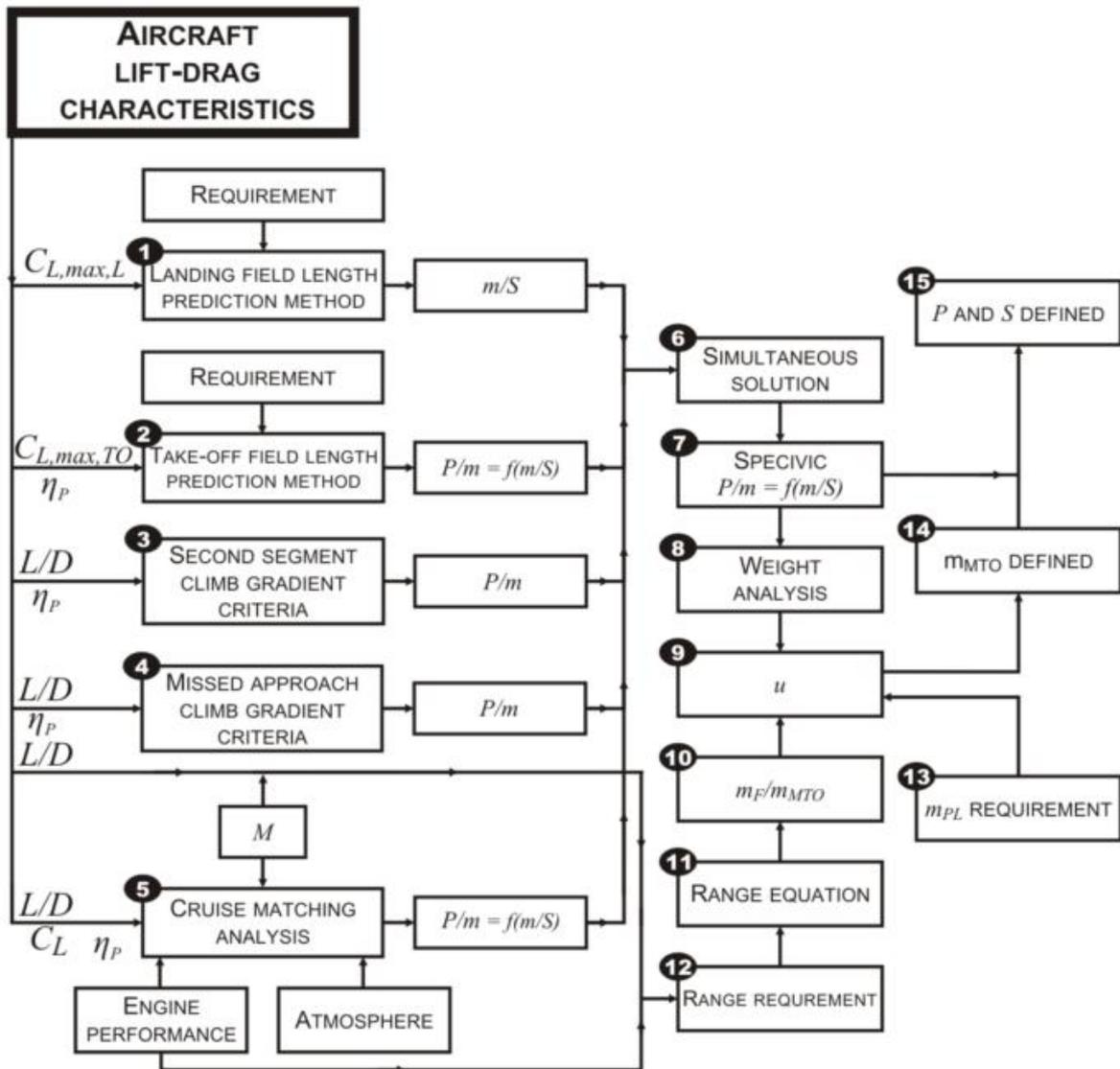
Figure 3: Overview of the preliminary sizing method for large propeller driven aeroplanes.
