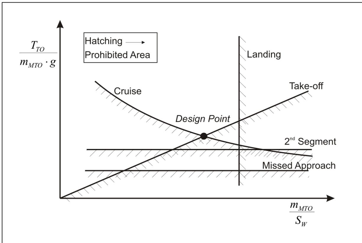
Figure 2: Hypothetical matching chart for a large jet aeroplane.
