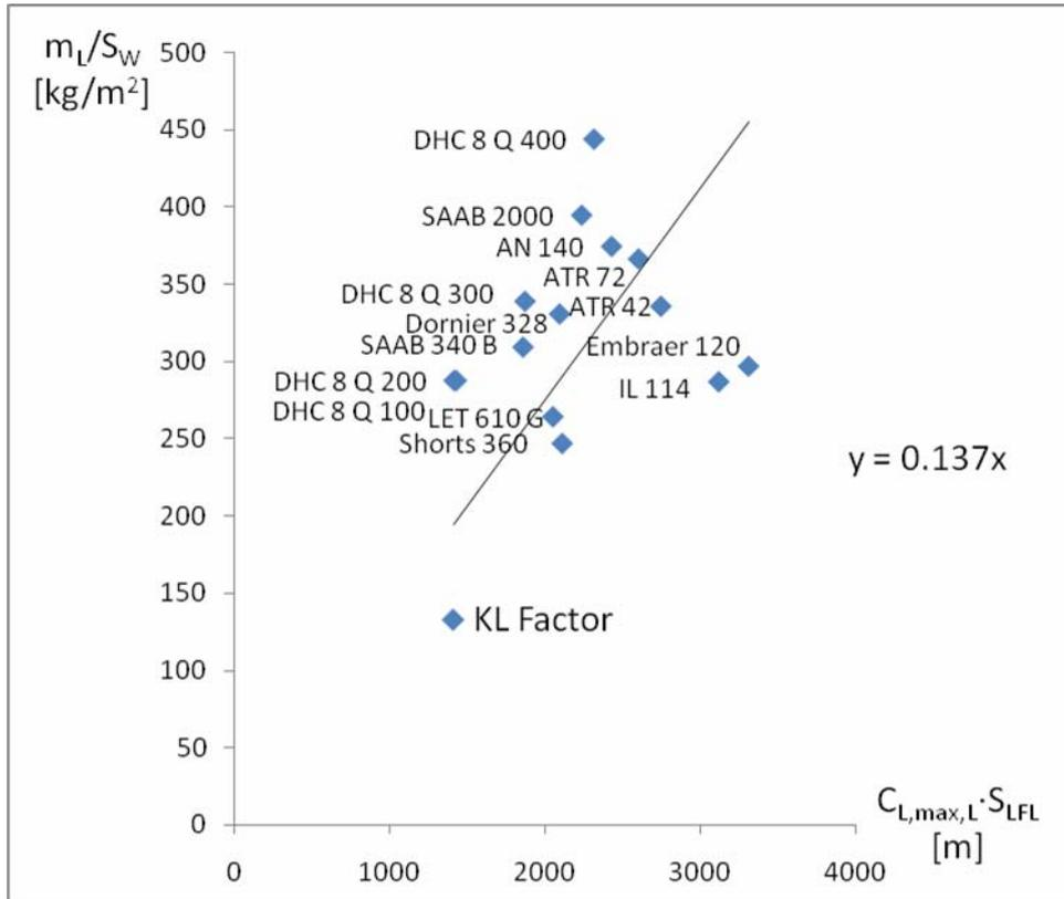
Figure 5: Statistical factor  $k_L$  for calculating wing loading from landing field length and maximum lift coefficient upon landing for turboprop aircraft.
