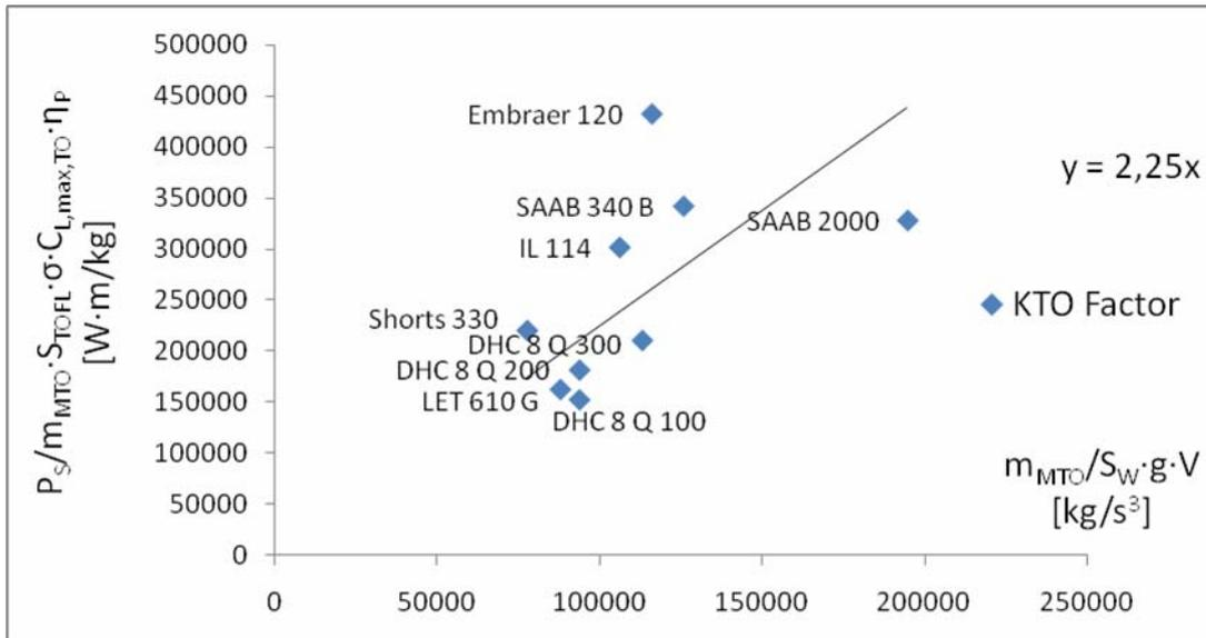
Figure 6: Statistical factor  $k_{TO}$  for calculating the take-off optimization parameter from take-off field length and maximum lift coefficient upon take-off for turboprop aircraft.
