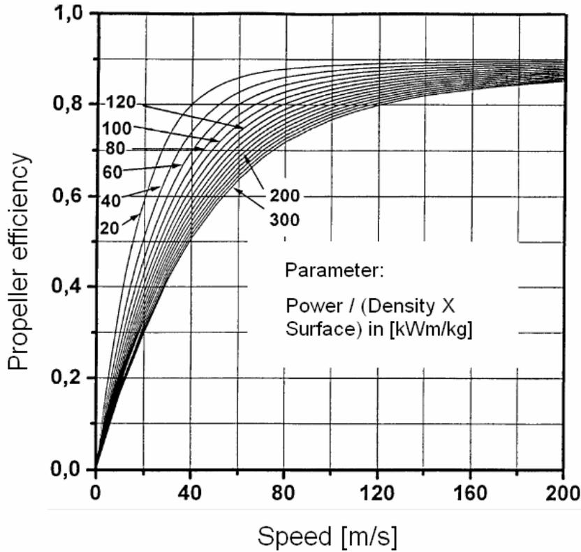
Figure 7: Propeller efficiency for variable pitch propellers as a function of aircraft speed and disc loading (the reference surface area is the propeller disc area). Adapted from [10]
