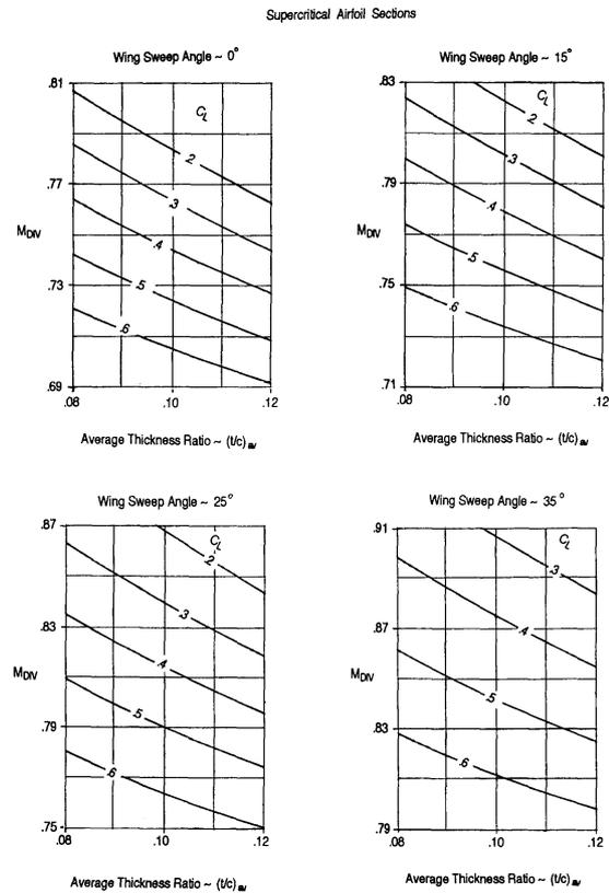
FIG 4. Determination of  $M_{DIV}$  or  $t/c$  from [10]
