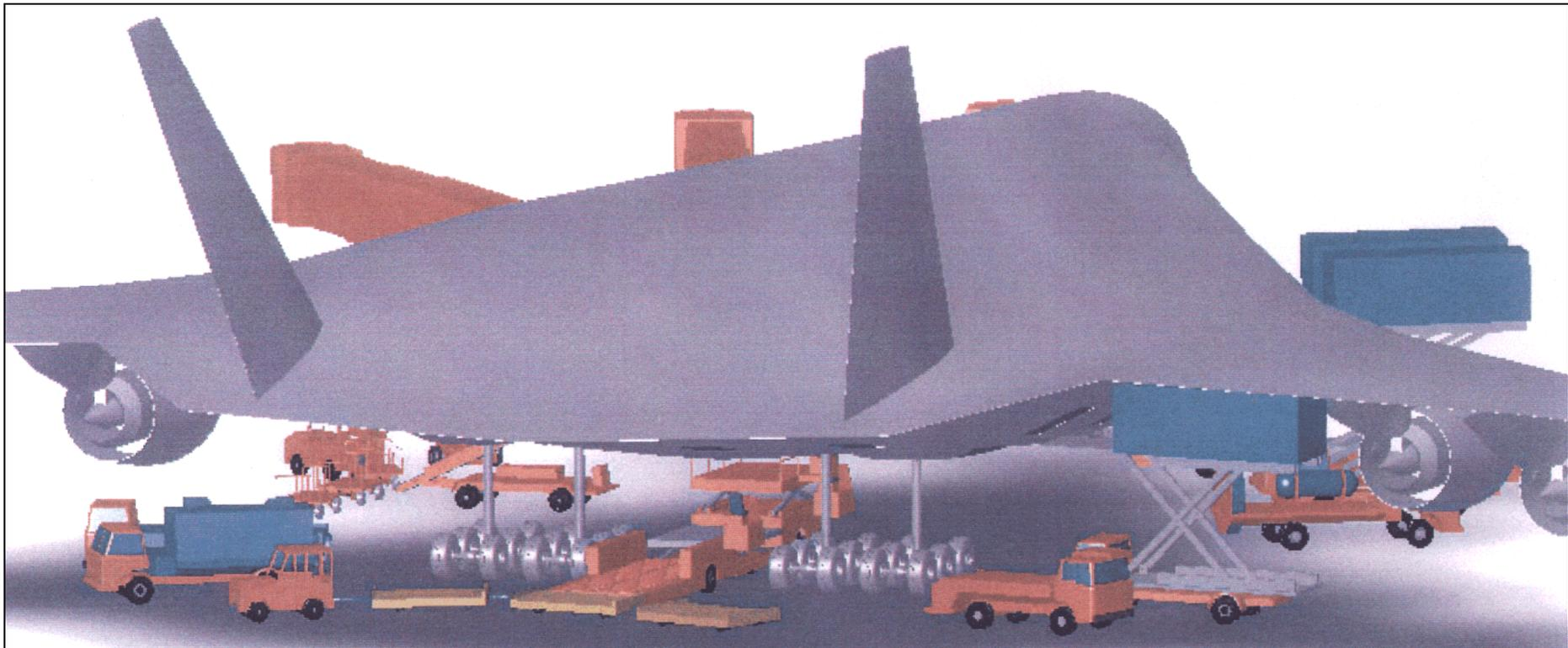
**A cargo loading vehicle drives in between the MLGs. Cargo loading from below with lifting system. Catering from the right.**
