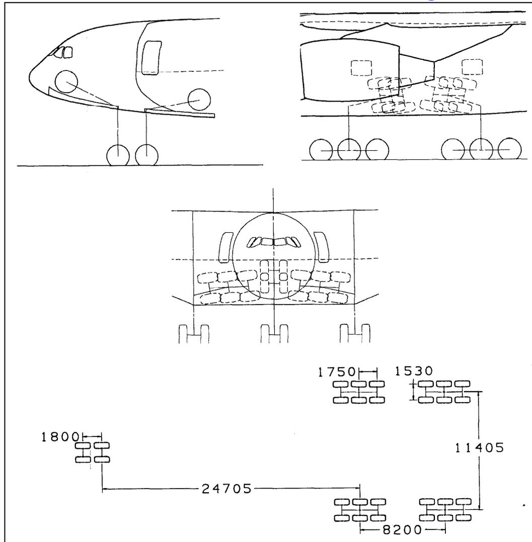
**Twin tandem (Bogie) nose landing gear.**
