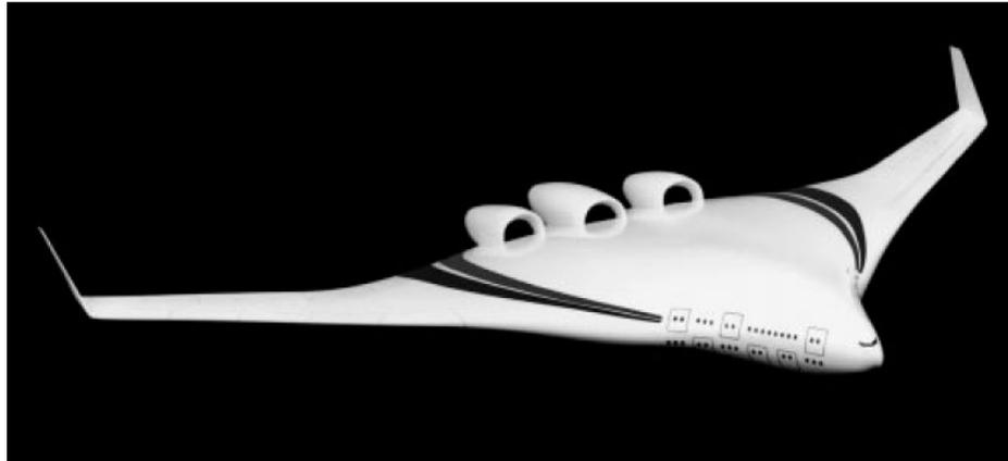
Blended Wing Body systems studies based on BWB-450 as part of the programme Ultra Efficient Engine Technology (UEET): Boundary Layer Ingestion (BLI) inlets with Active Flow Control (AFC).
