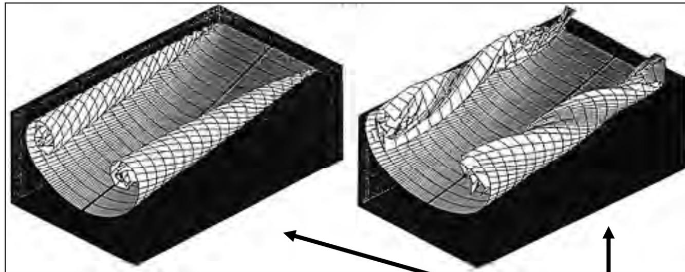
Decay of wake turbulence from a conventional wing and a C-wing.
