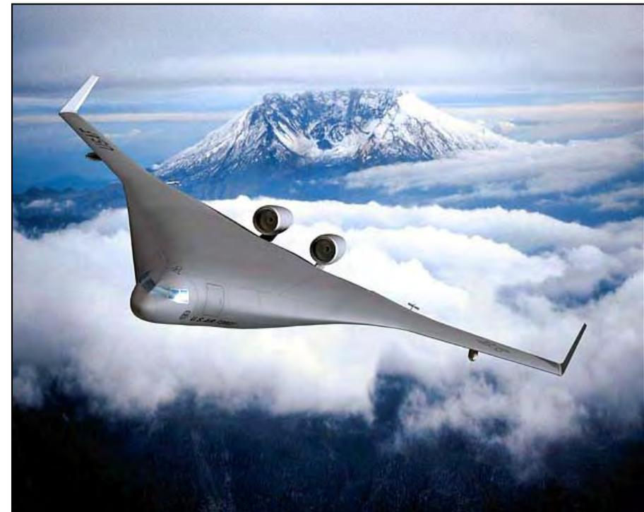
The X-48B prototypes have been dynamically scaled to represent a much larger aircraft.
