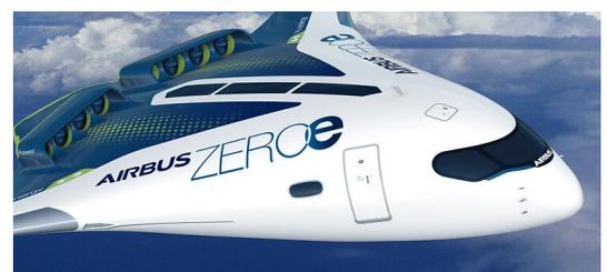
The aircraft has 8 engines. CS-25 defines the gradient of climb only up to 4 engines. The gradient is increasing with the number of engines. With many engines certification may require considering more than one engine inoperative. The chosen number of engines may have disadvantages based on certification rules, which however at this moment are not even given. This adds development risk.
