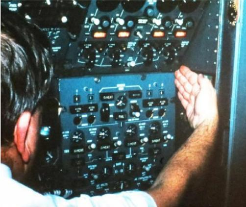
The flight engineer shows the gap that appears in flight between the instrument panel and the wall due to the fact that the aircraft got longer from the high skin temperature at Mach 2.
