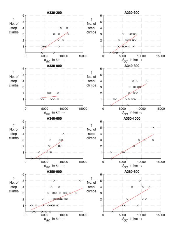
Figure 1: Number of step climbs relative to great circle distance of selected Airbus wide-body aircraft types
