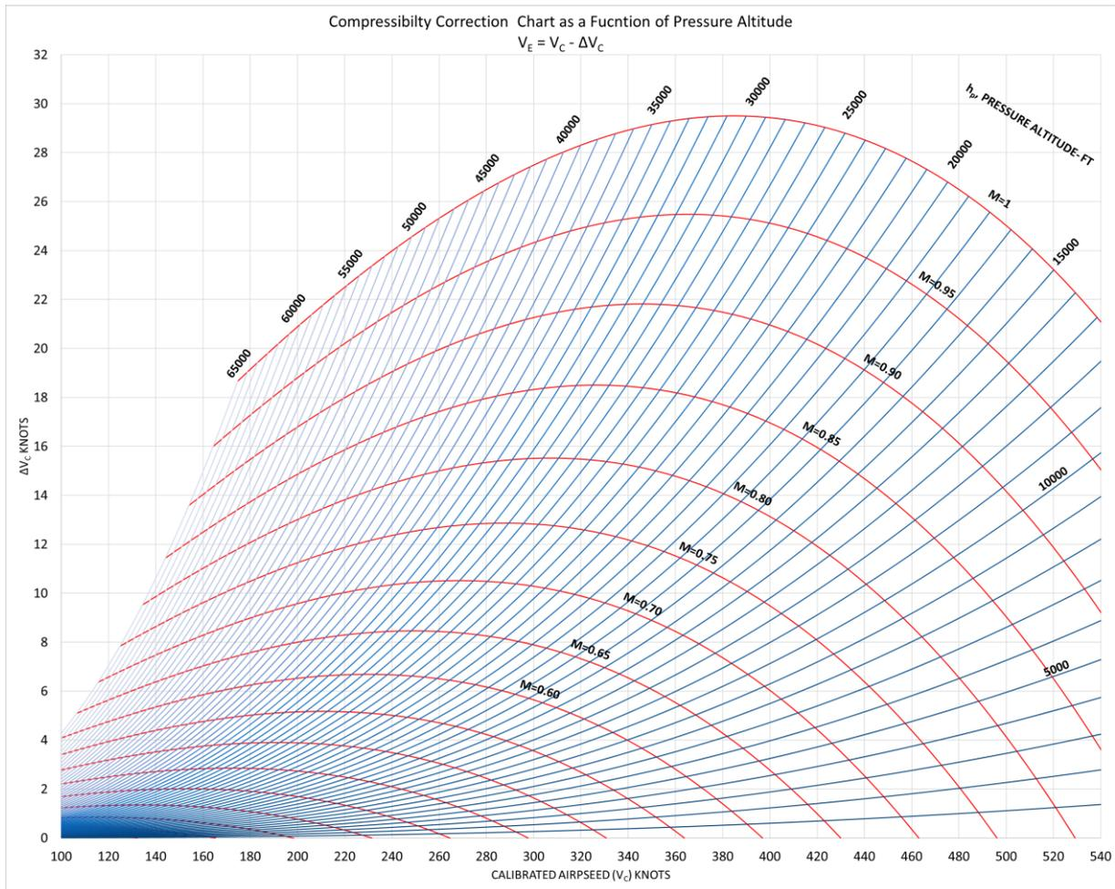
**Figure 1:** The Compressibility Correction Chart, converting from CAS to EAS.
