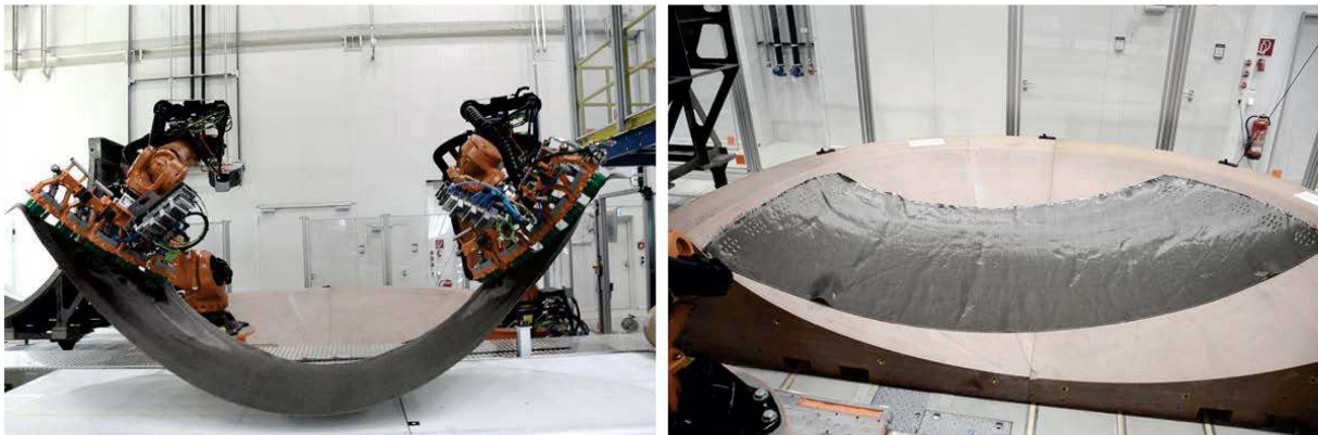
Figure 9: Transportation of the cut-piece (left), lay-up result (right)
