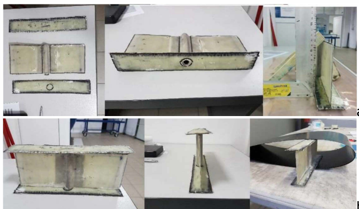
Figure 18. (a) The three components that assemblies the spar and (b) inserting the spar within the blade, near the leading edge
