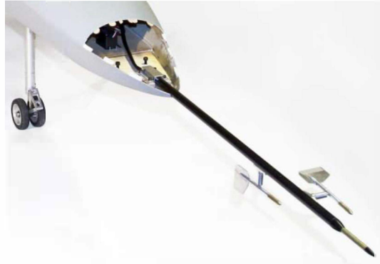
Figure 3: Direct measurement of the flow conditions improves significantly the flight reconstruction. Image shows a custom-made airdata nose-boom with alpha and beta transducers installed on the GFF platform.
