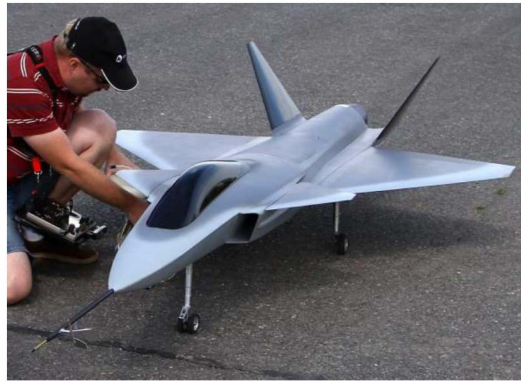
Figure 2: The GFF demonstrator: a 2-meter, jet-powered platform used for research at Linköping University [6].
