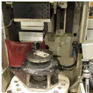
Figure 1 Arrangement of the sample and principles of ball on disk testing method.
