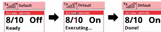
Figure 6: Information window of the custom Lua application for flight test, displaying the automatic execution of a test point. The screenshots are extracted from the main screen of the pilot's transmitter, in this case a Jeti Model DC-24 [13].
