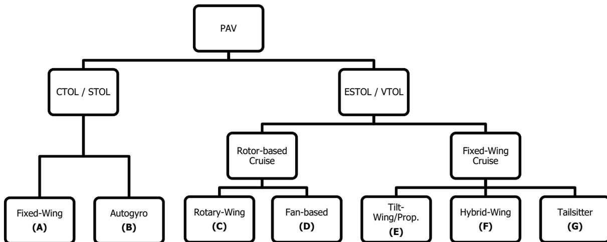
**Figure 1: PAV classification scheme regarding take-off/landing capability and vehicle morphology**
