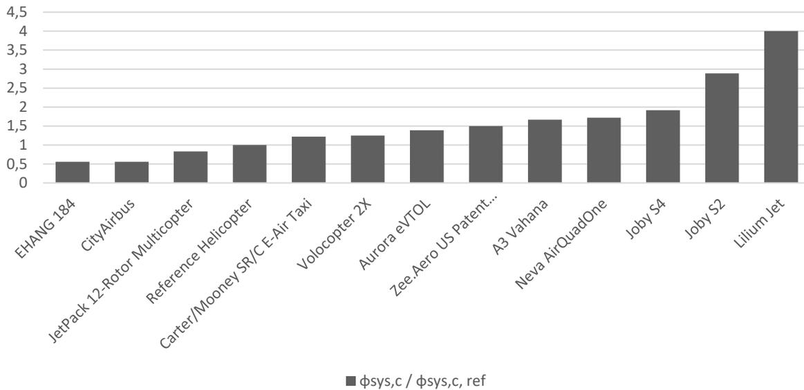
**Figure 16: Normalized coupled system complexity of fully-electric VTOL PAV configurations.**
