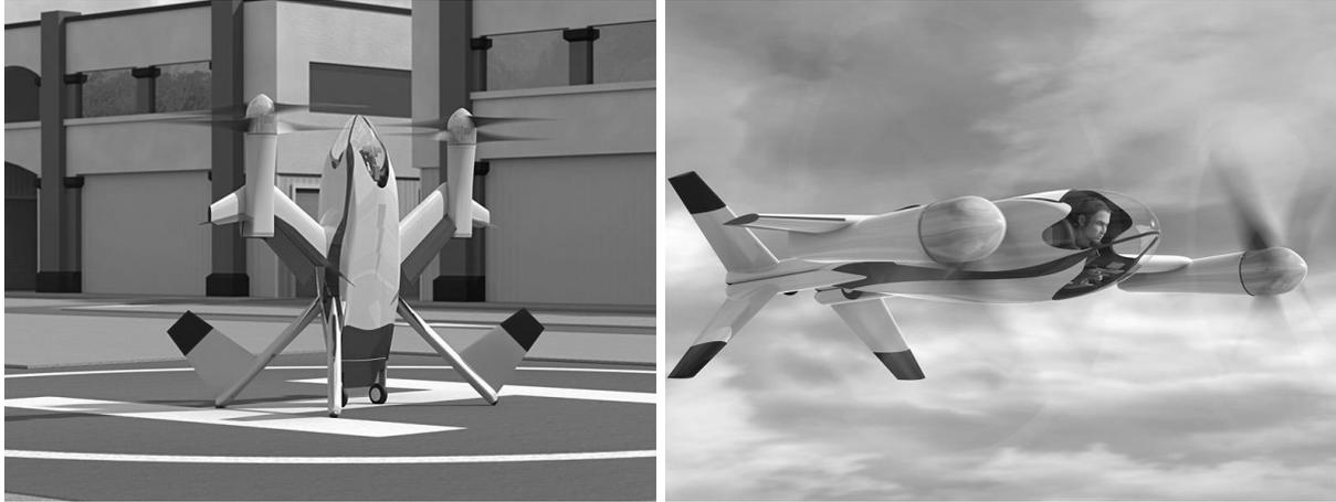
**Figure 11: Illustrations of the NASA "Puffin" tailsitter configuration on ground in upright position (left) and during horizontal flight (right) [67].**
