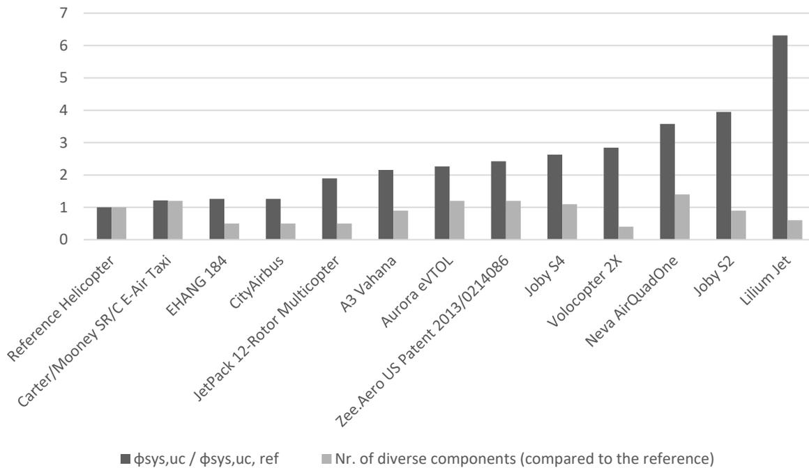
**Figure 15: Normalized uncoupled system complexity and number of diverse components of fully-electric VTOL PAV configurations.**
