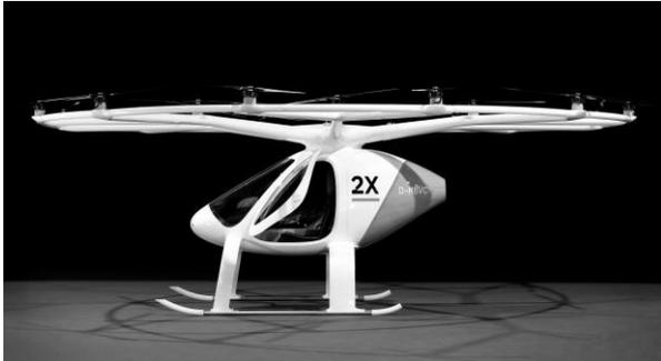
**Figure 2: Volocopter's two-seated series model 2X lifted by 18 rotors [24].**
