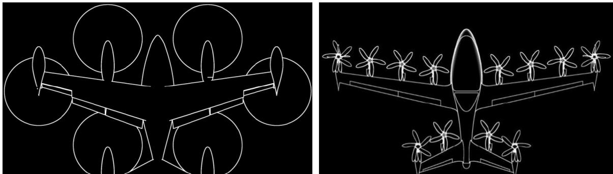
**Figure 6: Top view of the Joby S4 (left) and the S2 (right) tilt-propulsor PAVs with foldable propellers [38].**
