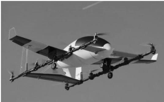
**Figure 9: Aurora eVTOL hybrid-wing subscale prototype [51].**
