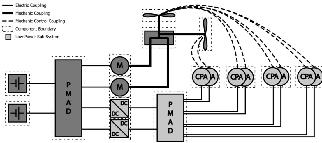
**Figure 14: Reference power train and flight control system of a full-electric helicopter.**
