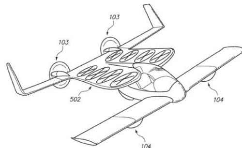
**Figure 10: Zee.Aero patent figure of a hybrid-wing configuration, fitting in a standard car parking lot [50].**
