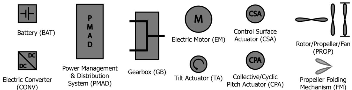
Figure 13: Abstract assembly parts of power trains and flight control systems
