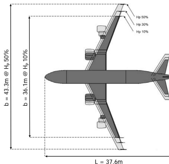
**Figure 2: Top view of the year 2035 the discrete parallel hybrid-electric derivative for different degrees of power hybridization [10]**
