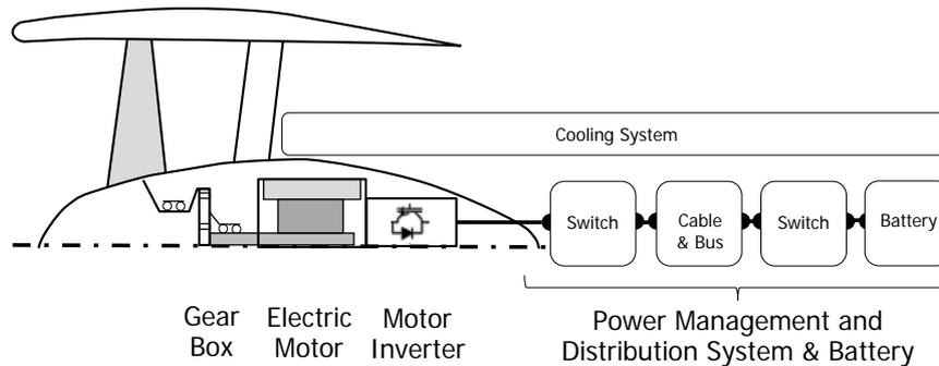
Figure 3: Typical components required for an electrically powered ducted fan
