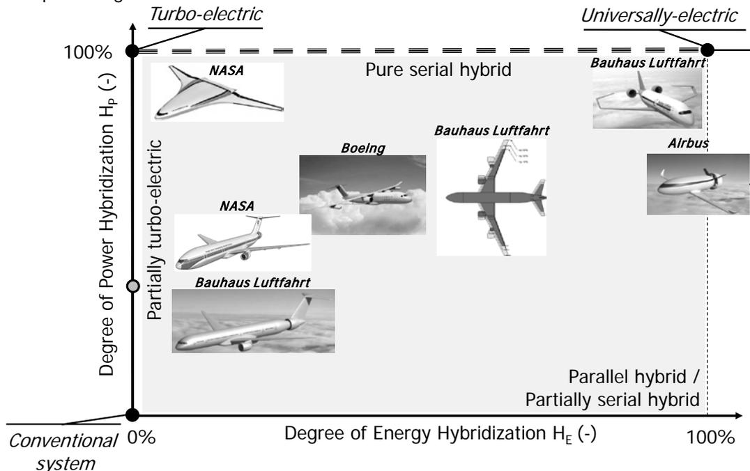
**Figure 1: Various turbo-, hybrid- and universally electric concepts marked in the degree of power and energy hybridization diagram for battery-kerosene hybrid-electric aircraft**
