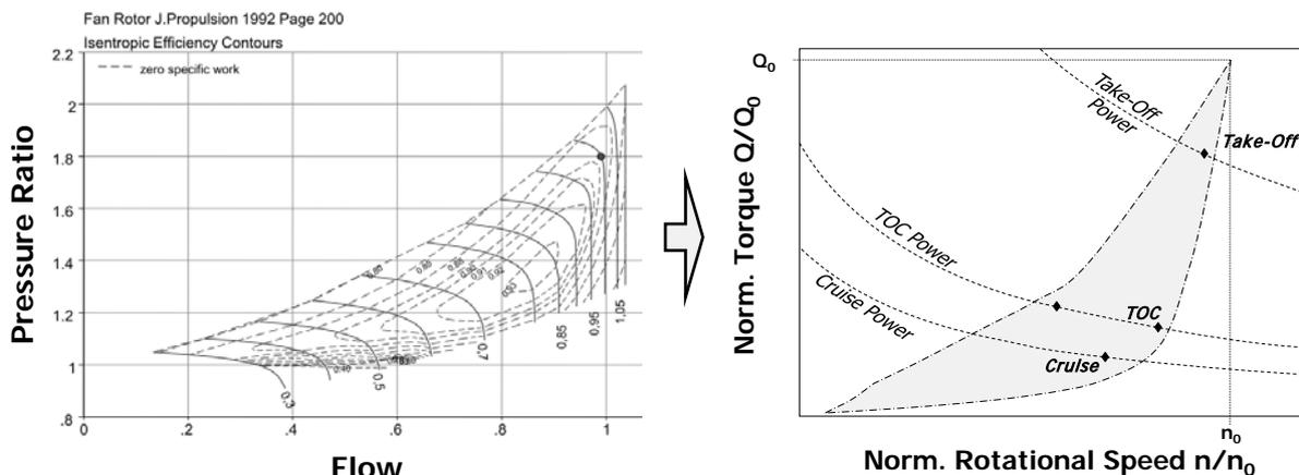
**Figure 7: Conventional fan map as function of pressure ratio and mass flow (left) [21]; transformed generic fan map as a function of rotational speed and shaft torque (right)**
