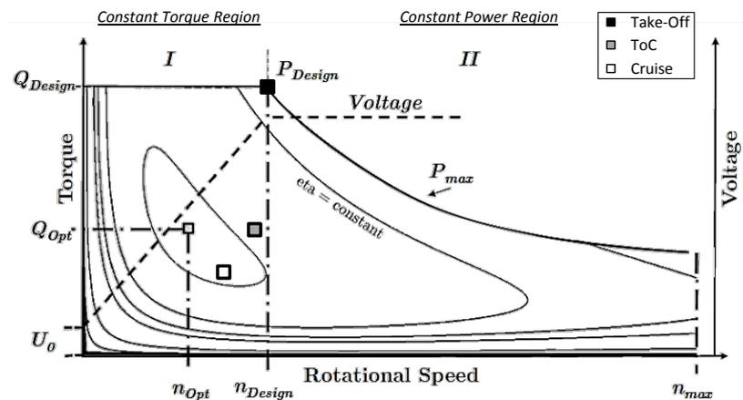
**Figure 5: Generic performance chart of an electric motor based on [14]**
