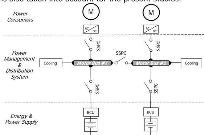
Figure 4: Main components of a battery supplied electric systems architecture design with two separated propulsion chains in normal operation
