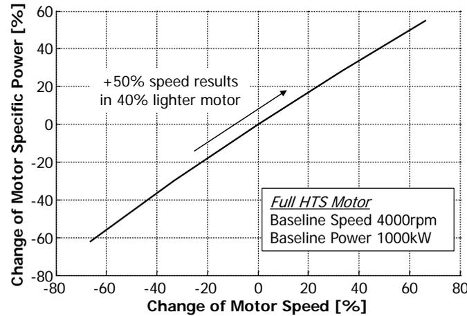
**Figure 6: Impact of the rotational speed on the electric motor mass (without cooling and inverter)**
