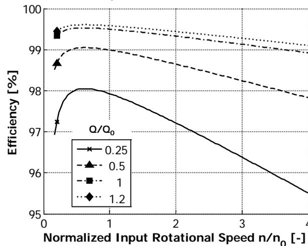
**Figure 8: Normalized off-design performance of a single stage planetary gear box based on [23]**
