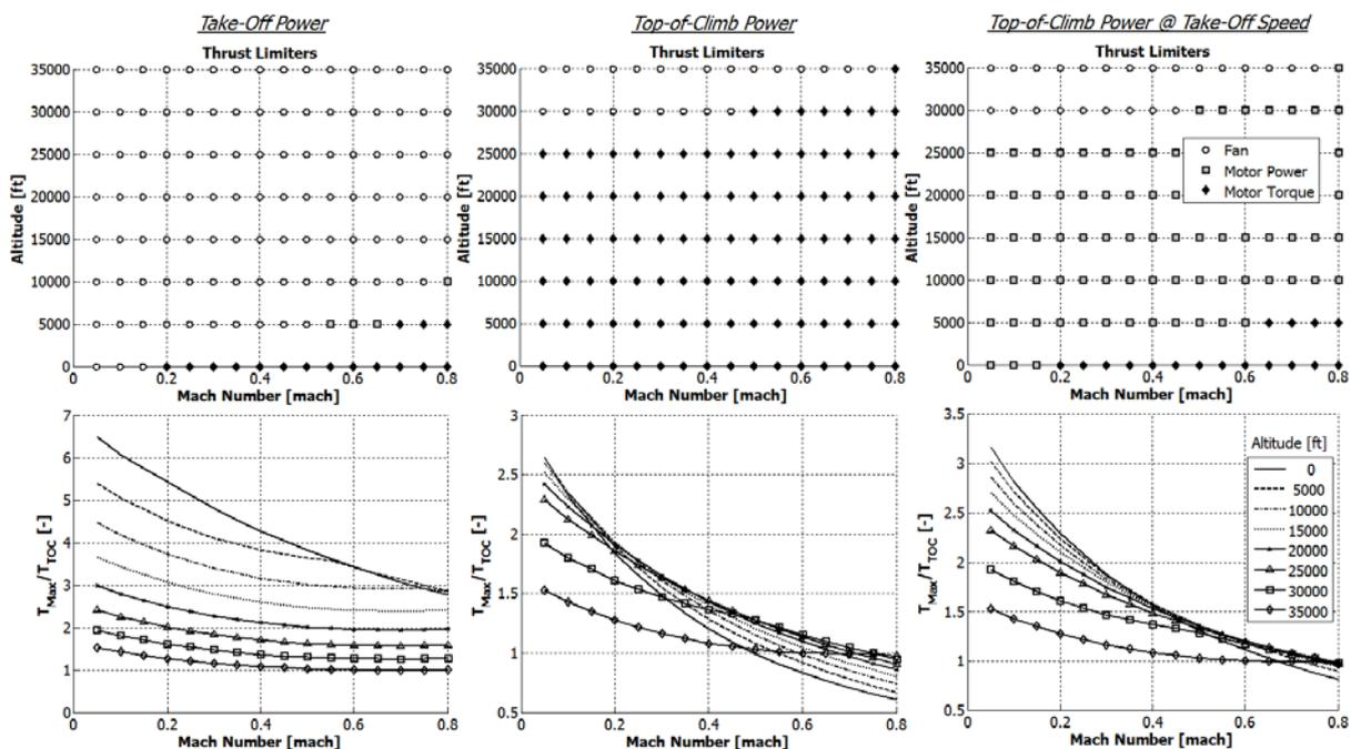
Figure 11: Thrust limiting parameters (top) and maximum available thrust (bottom) based on top-of-climb thrust for different motorization options
