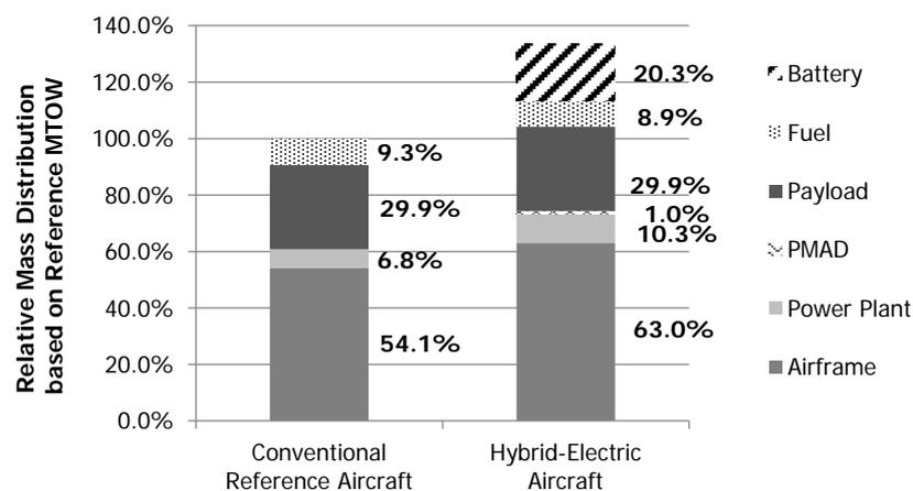
**Figure 12: Comparison of the reference aircraft with the discrete parallel hybrid-electric aircraft for 1300nm and a battery specific energy assumption of 1000Wh/kg**
