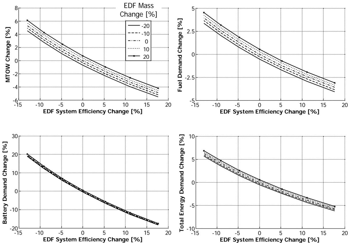
**Figure 13: Sensitivity results by changing the overall EDF system efficiency and mass to identify the impact on the MTOW and total energy demand for Sizing No. 3 at  $H_p$  30%**
