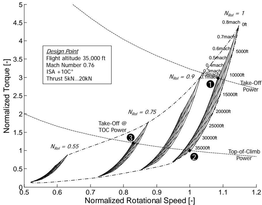
Figure 10: Normalized rotational speed and torque diagram of the ducted fan model at different thrust lever positions (normalized to TOC conditions)
