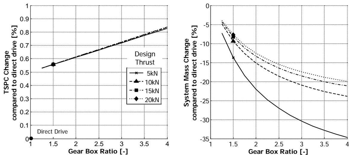
Figure 9: Impact of the design gear ratio on the system efficiency (left) and mass (right)
