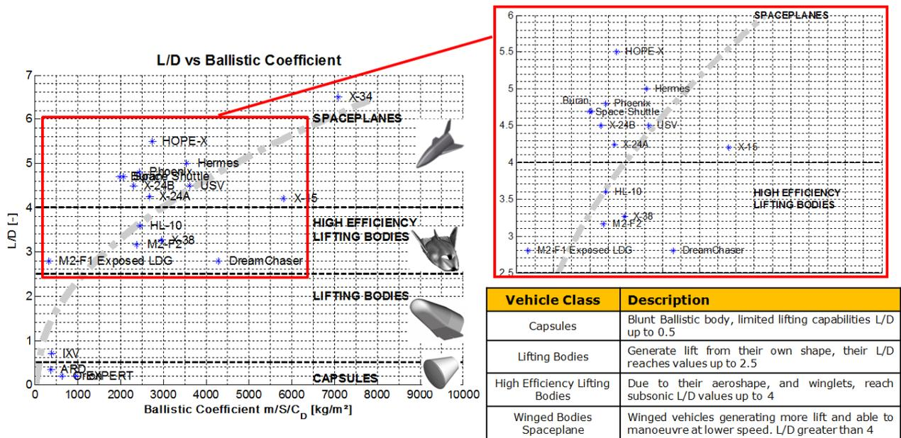
Figure 1: State of art of entry solutions according to the identified vehicle classes
