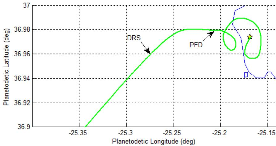
Figure 10: End-2-end Reference trajectory ground track, final TAEM and Descent phases
