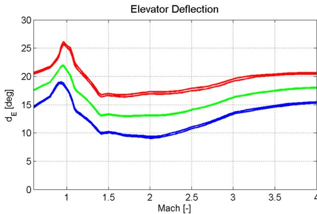
Figure 7: FQA Trimline Elevator Deflection performance versus Mach for the REVLANSYS vehicle, TAEM phase (0.5%tile-blue, 50%tile-green, 99.5%tile-red)
