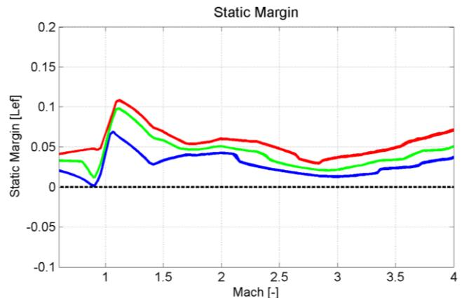
Figure 8: FQA Trimline Static Margin performance versus Mach for the REVLANSYS vehicle, TAEM phase (0.5%tile-blue, 50%tile-green, 99.5%tile-red)
