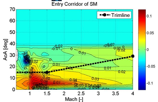
Figure 6: FQA Nominal Trimline and Static Margin performance for the REVLANSYS vehicle, TAEM phase
