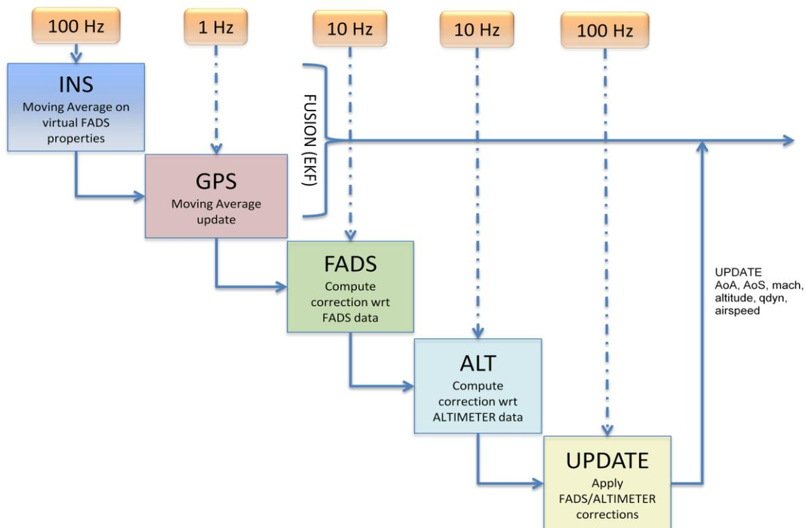
Figure 21 Navigation architecture with loosely coupled INS/GNSS and uncoupled FADS and altimeter
