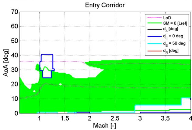
Figure 5: FQA AoA-Mach Entry Corridor (indicated in green) of the REVLANSYS vehicle, TAEM phase
