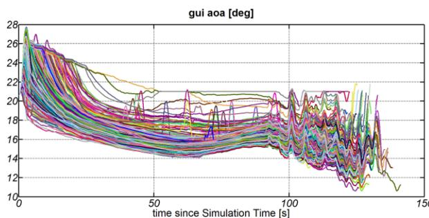
**Figure 25 Commanded Angle of Attack during TAEM**
