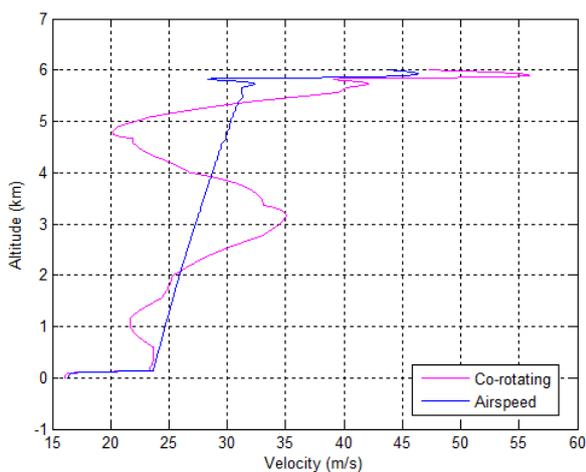
Figure 12: Reference trajectory velocity profiles, Descent under parafoil
