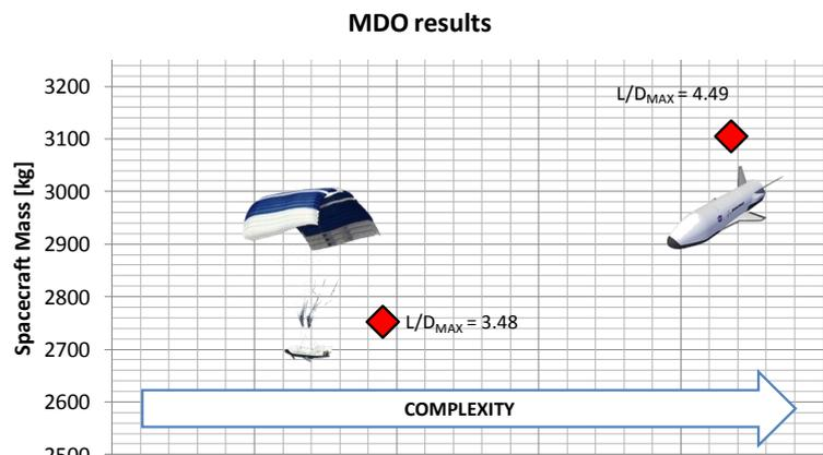
Figure 3: Optimised preliminary design solutions with example aeroshapes
