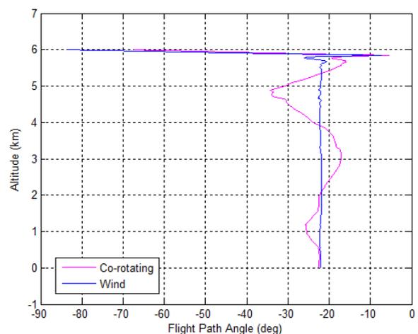
Figure 13: Reference trajectory flight path angle profiles, Descent under parafoil
