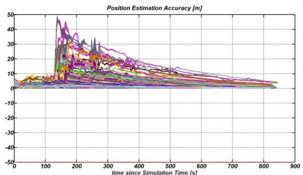
**Figure 26 Position estimation accuracy from TEP to touchdown**
