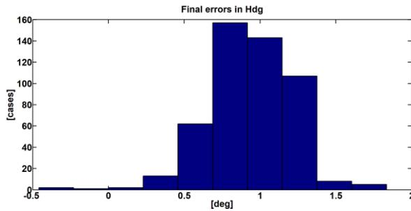
**Figure 27 Heading accuracy at TDW (Open Loop Trajectory Generation test)**
