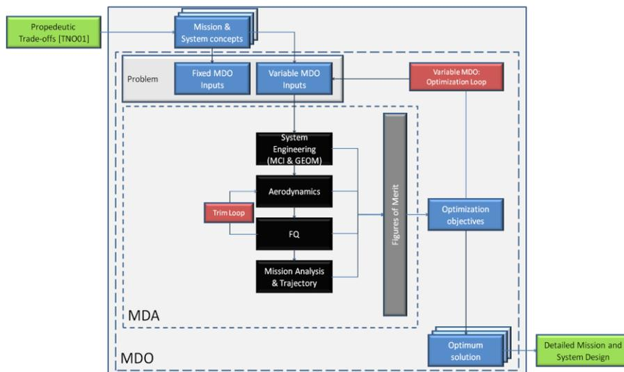
Figure 4: MDA-MDO design process for REVLANSYS.
