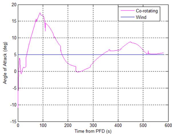
**Figure 14: Reference trajectory angle of attack profiles, Descent under Parafoil**
