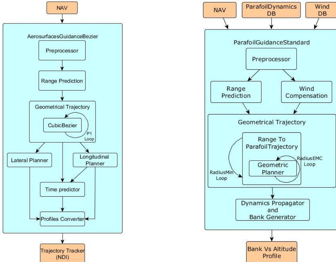
Figure 20 Aerosurfaces Guidance architecture [left], Parafoil Guidance Architecture [right]
