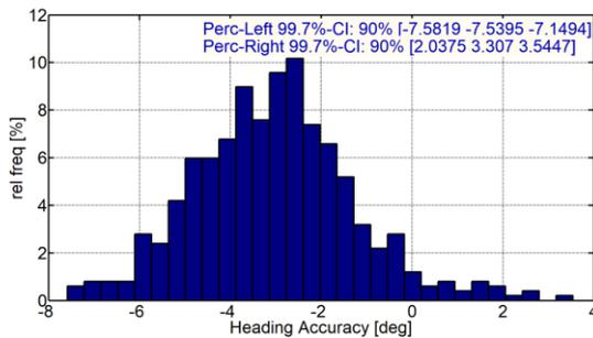
**Figure 23 Heading accuracy at the end of TAEM**
