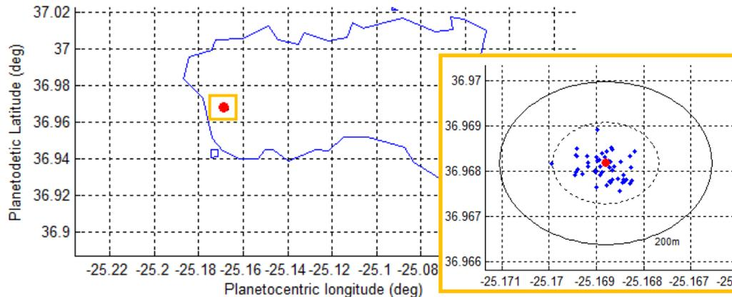
**Figure 29 Touchdown accuracy (Closed Loop Parafoil Guidance test)**
