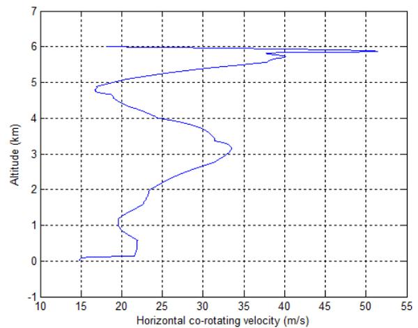
**Figure 15: Reference trajectory horizontal velocity wrt ground profile, Descent under Parafoil**
