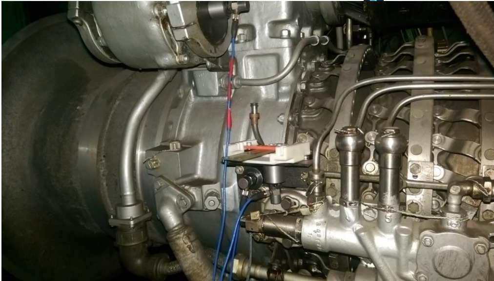
Figure 19: Position of the harvester and accelerometers
