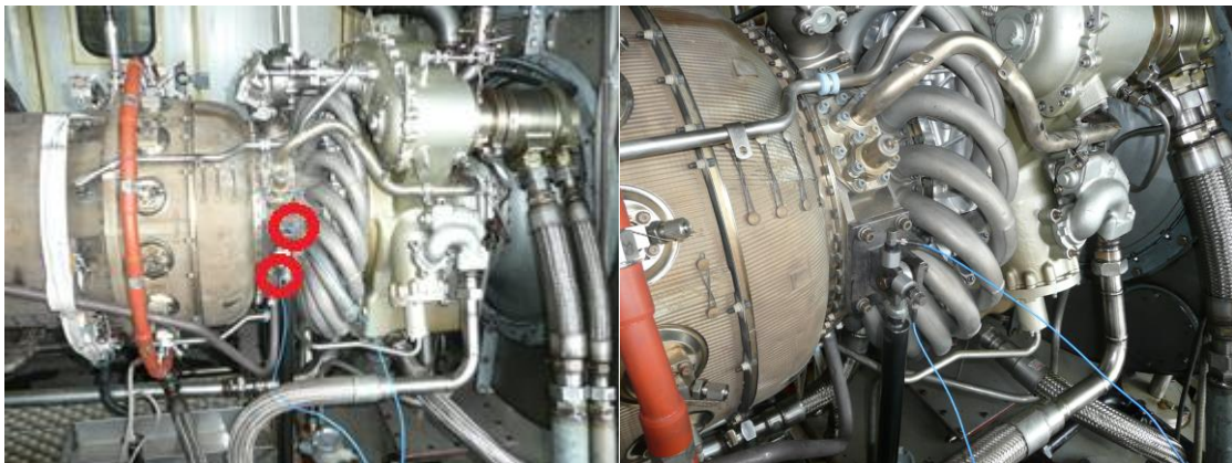
Figure 13: Vibration measurement on the ST18 engine
