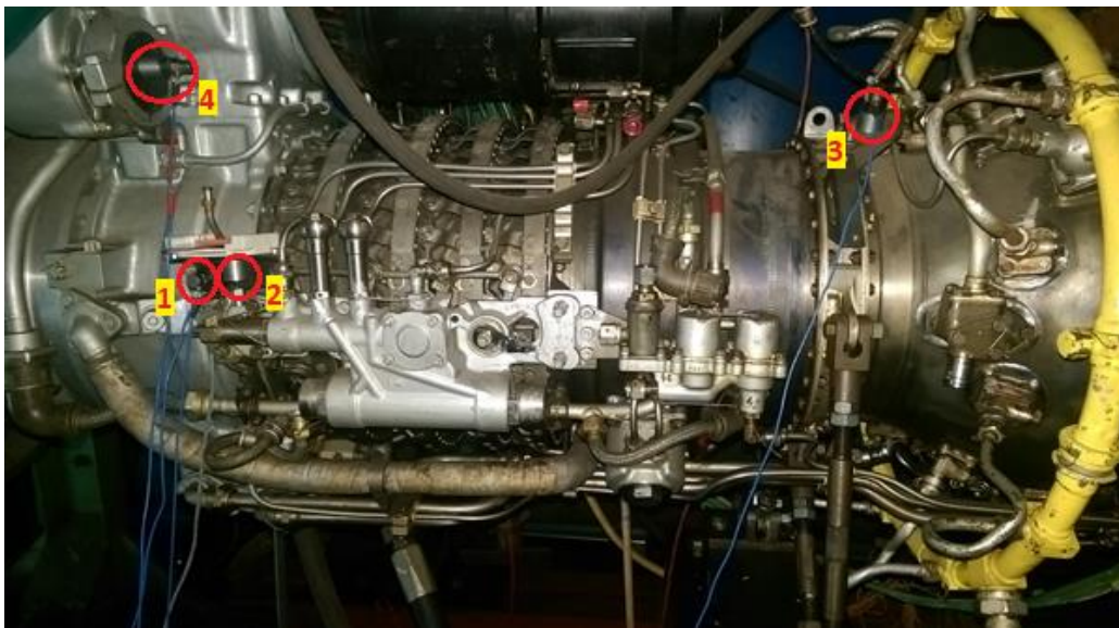
Figure 20: Position of the harvester and accelerometers along the engine: (1) axial-horizontal near the harvester, (2) axial-vertical near the harvester, (3) at the end of the compressor, (4) on the engine starter
