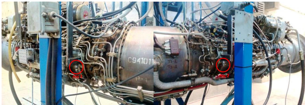
Figure 10: Vibration measurement on two TV2 engines
