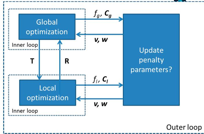
**Figure 4: Sequential update process of the subsystems optimizations.**
