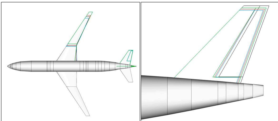
**Figure 14: Wing planform (left) and VTP (right) comparisons of optimal designs: 1-blue, 2-red, 3-green (with increasing wing span) versus the baseline configuration (black).**
