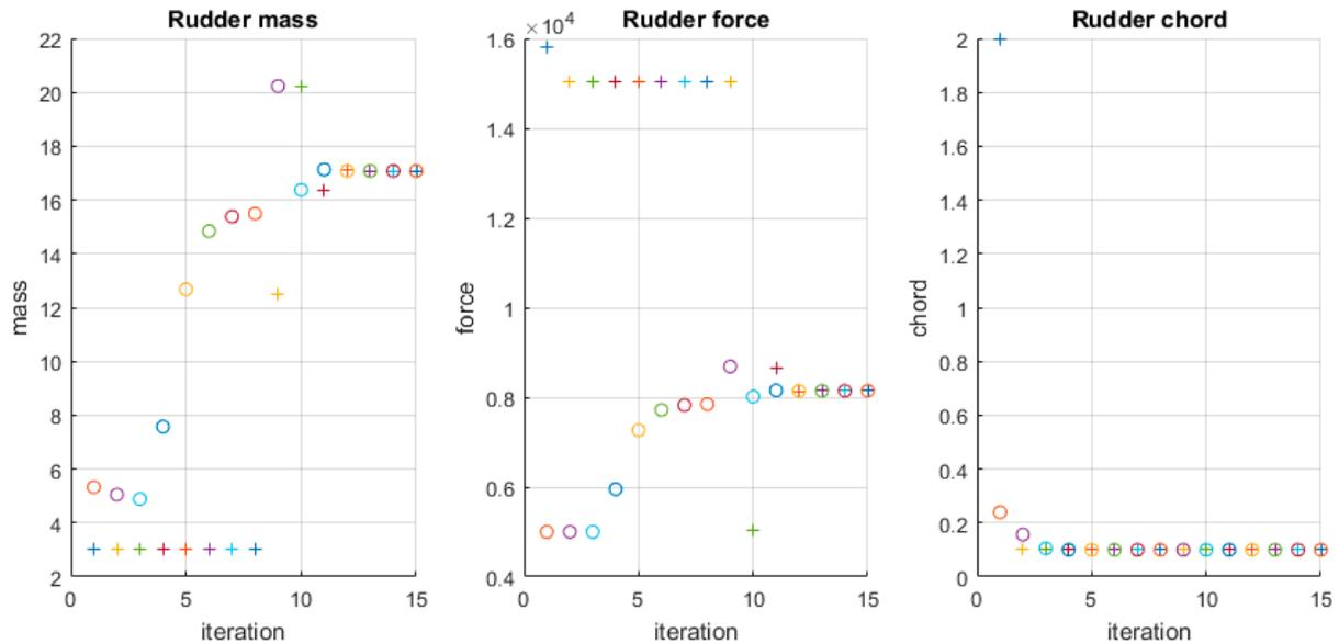
**Figure 5: MLO outer loop iterations of coupling variables. The + signs represent the globally optimized values (targets). The o signs represent the locally optimized values (responses).**
