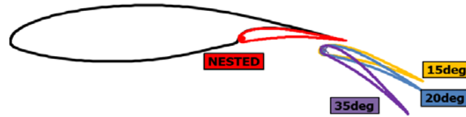
Figure 12: Fowler flap design for the kink section, flap chord length is 0.32% of chord.
