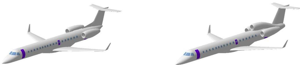
**Figure 2: Twin-jet and trijet configuration**
