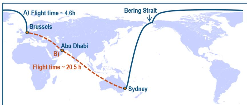
**Figure 2: Representative flight trajectories for the baseline mission Brussels to Sydney of the EU-funded LAPCAT study [39] for a route with A) hypersonic cruise (at Mach 5) and B) the conventional subsonic reference.**
