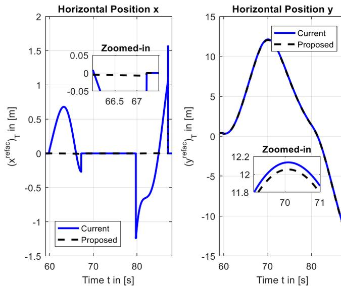
**Figure 4: Comparison of horizontal position deviations of current and proposed method.**
