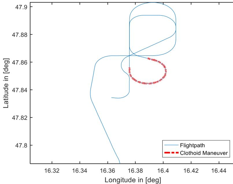
**Figure 8: Aircraft flight path with marked clothoid manoeuvre.**
