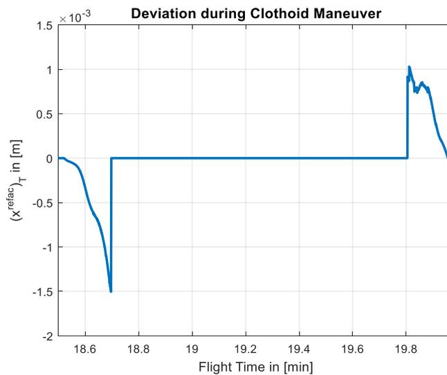
**Figure 9: Horizontal position deviation during the radius-to-fix clothoid manoeuvre.**
