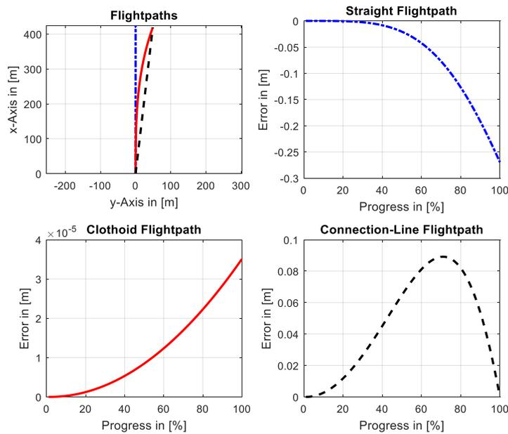
**Figure 6: Error in reference point projection of local tangent for straight line (dashed-dot blue), clothoid (solid red), and connection line (dashed black) flight of the aircraft.**
