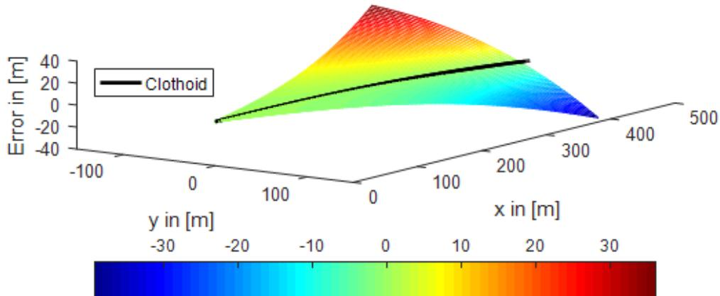
**Figure 7: Error in reference point projection for multiple straight line flight paths from the clothoid start around a reference clothoid.**
