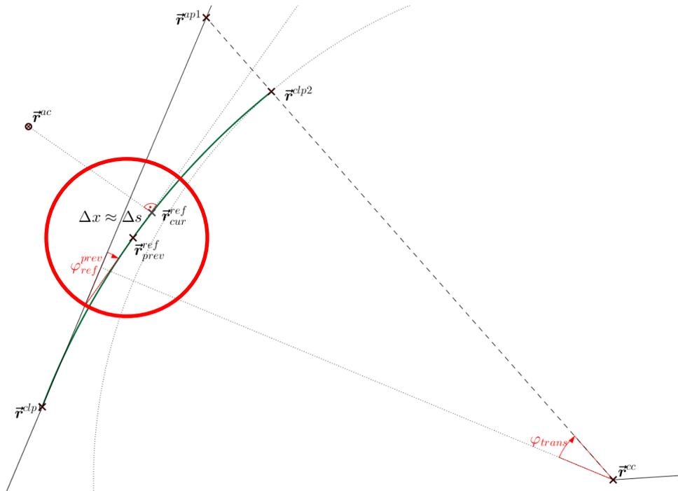
**Figure 3: Proposed procedure for reference point calculation by projection on tangent of the previous clothoid reference point.**
