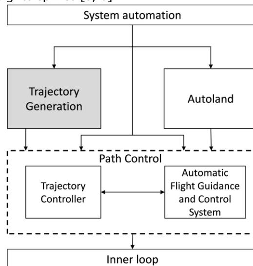
**Figure 1: Structure of integrated mission management system of the CS-23 aircraft [2].**
