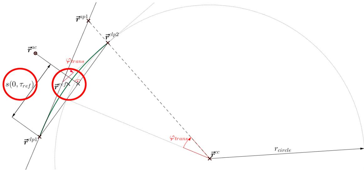
**Figure 2: Current procedure for reference point calculation by projection on connection line between clothoid starting and ending point [1].**
