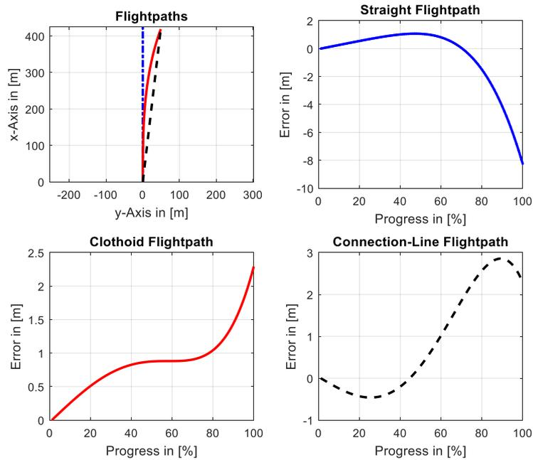
**Figure 5: Error in reference point projection of connection line for straight line (dashed-dot blue), clothoid (solid red), and connection line (dashed black) flight of the aircraft.**
