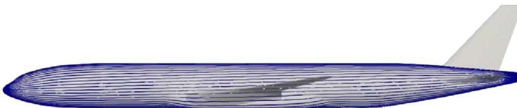
Figure 6: Stringer extrusion paths for linear interpolation scheme
