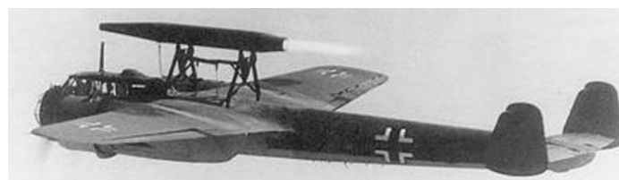
Figure 6: Ramjet test flight on Do-17
