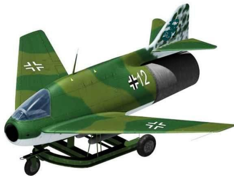
Figure 7: "Škoda-Kauba Sk P.14" fighter project [13] with Dr. Eugen Sänger's ramjet
