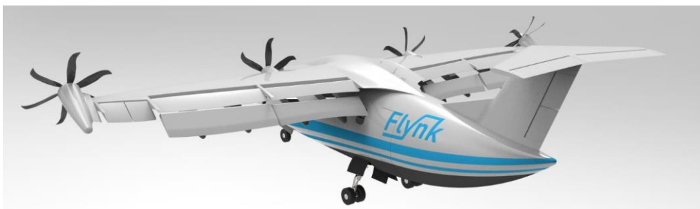
Figure 8: Flynk's fully-extended flap configuration.
