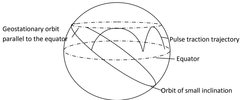
Figure 1: The pulse traction trajectory of the satellite
