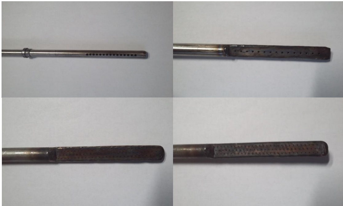
Figure 4: The 4 tested injection nozzles
