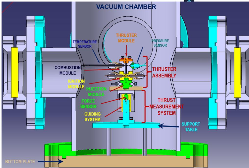
**Figure 5: Thruster experimental assembly – section view details**
