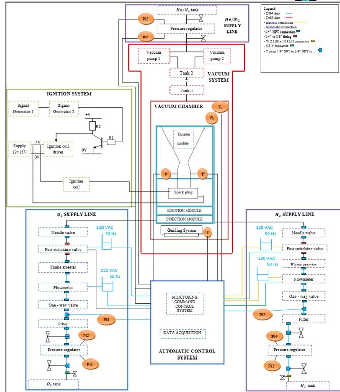
Figure 3: Experimental installation - Main systems
