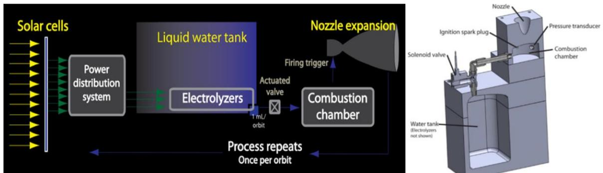
Figure 2: Schematic of the operation of a CubeSat prototype electrolysis propulsion system
