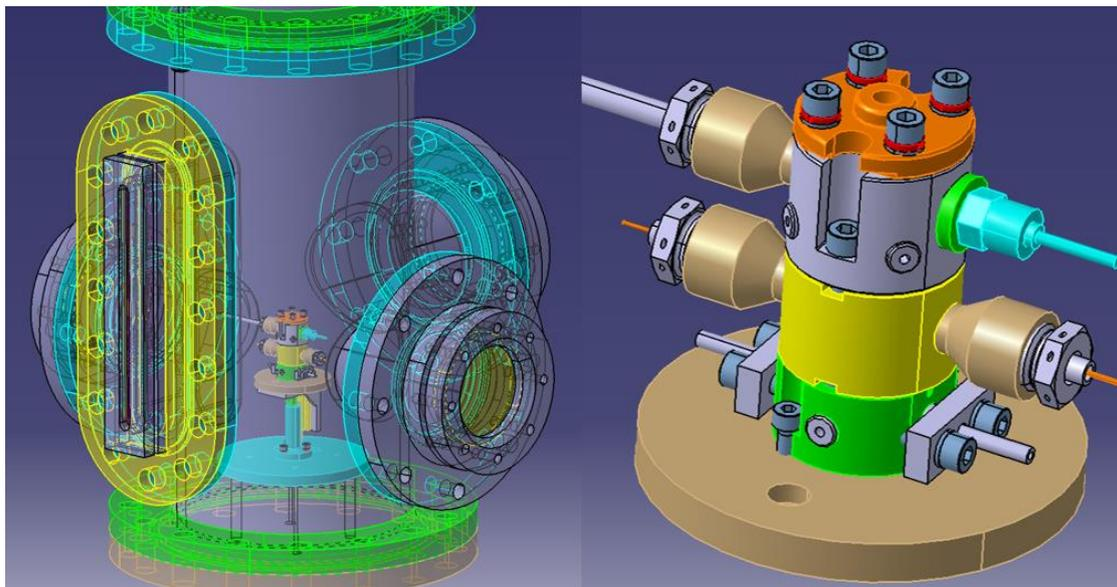
Figure 4: Thruster experimental assembly inside the vacuum chamber
