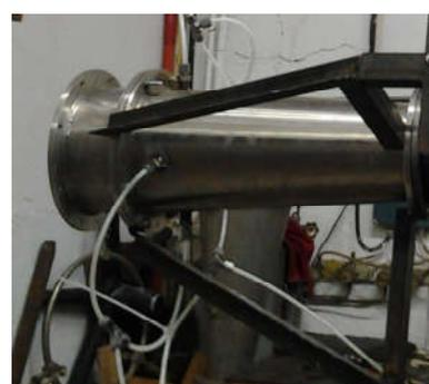
Fig. 5 Temperature probe, static probes placement on the secondary air stream inlet and at jet pump exit
