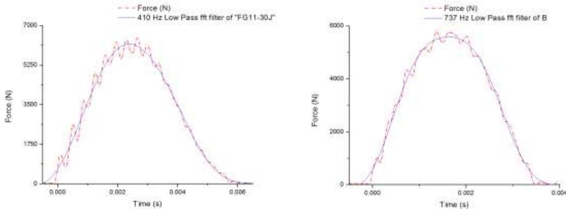
**Figure 5 - Comparison between the as acquired and low pass filtered curves.**
