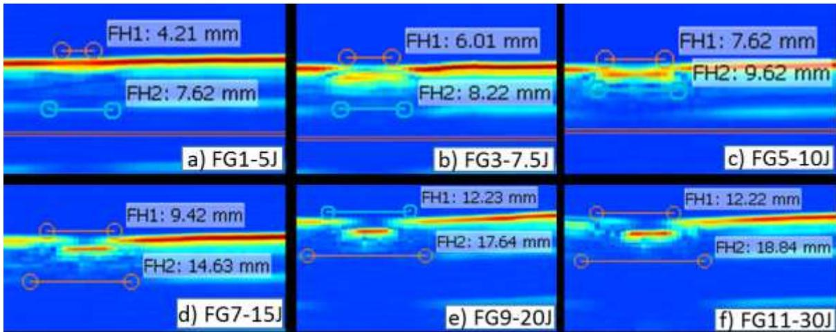
**Figure 3 - Damage characterization B-Scans – Glass Fibre - 5J to 30J (a-f).**
