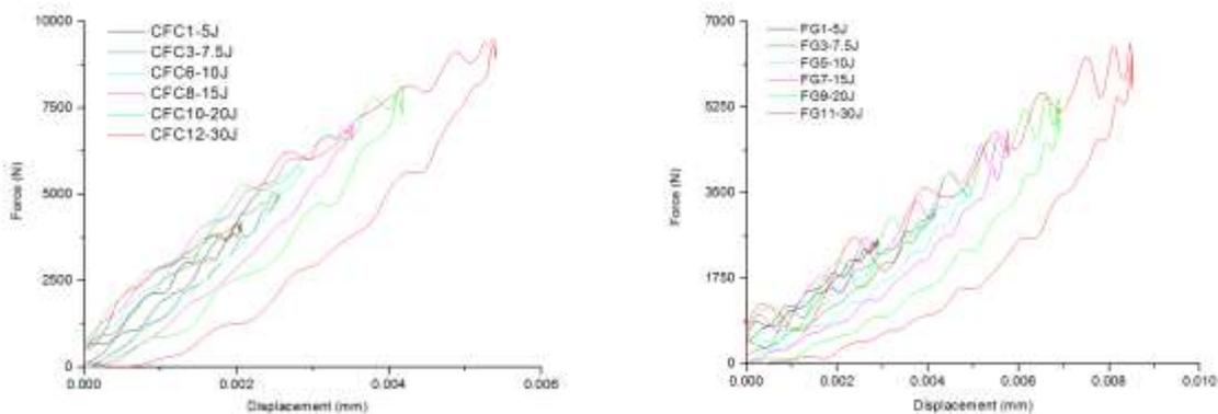
**Figure 6 - Force displacement curves for carbon fibres (left) and glass fibres (right).**
