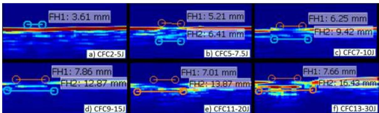
Figure 2 - Damage characterisation B-Scans – Carbon Fibre - 5J to 30J (a-f).
