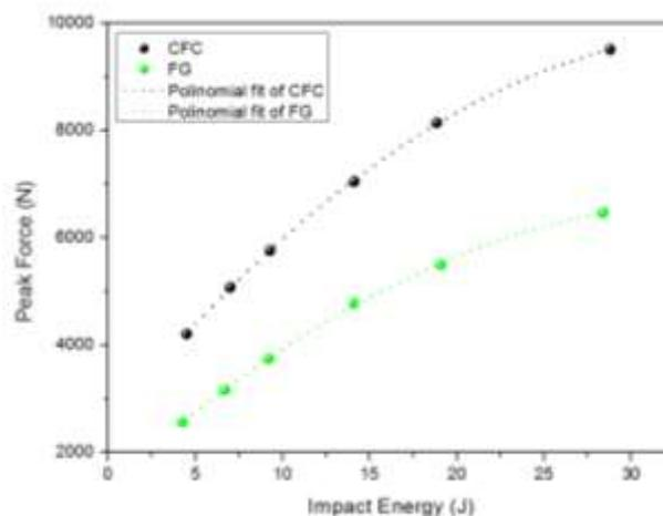
**Figure 8 - Peak force as a function of the impact energy for the carbon fibres (black) and glass fibres (green).**
