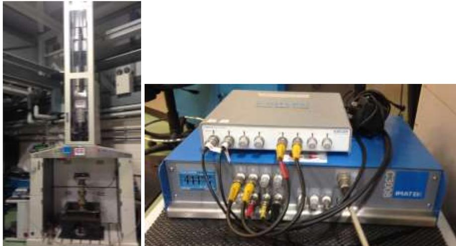
Figure 1 - Drop tower and details of the acquisition system used for the testing.
