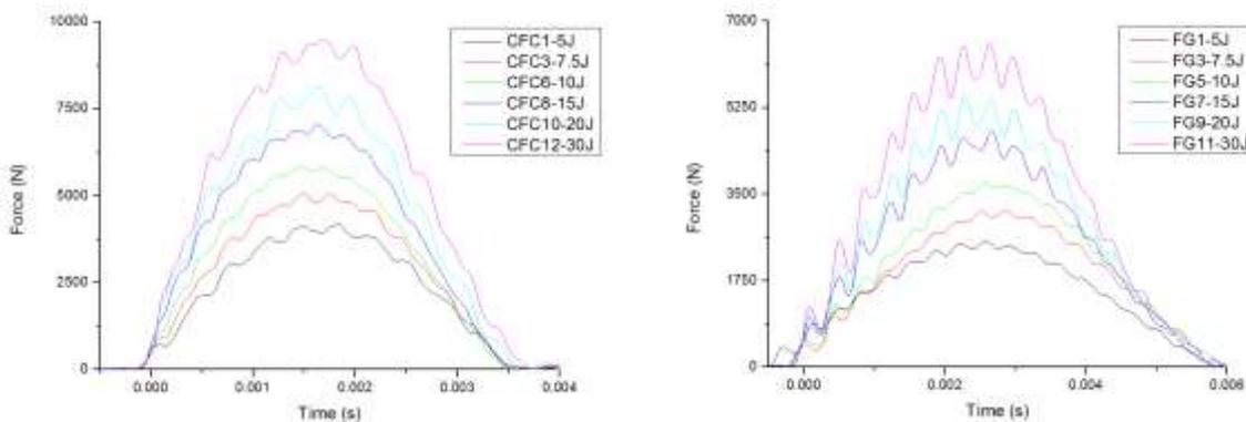
**Figure 4 - Force time history for Carbon (left) and Glass (right) fibres tested.**
