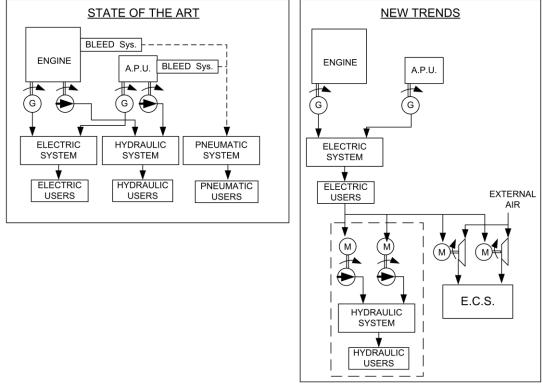
Figure 3: State-Of-The-Art and New trends On-Board systems architectures.
