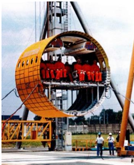
Figure 1: Scale 1 crash test at DGA TA (1995) – EU TIM-Crash project
