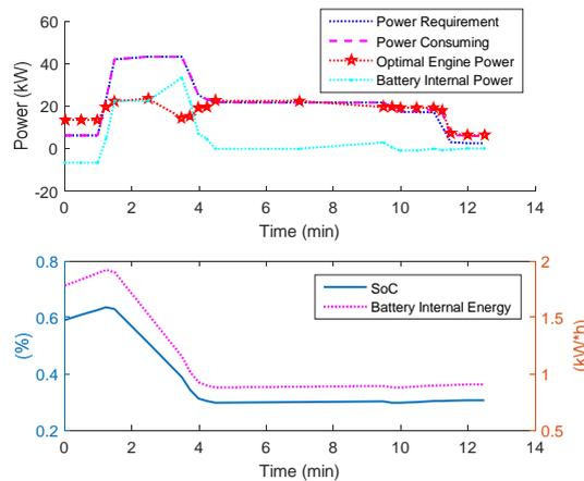
**Figure 6. Optimization results of test case 1.**
