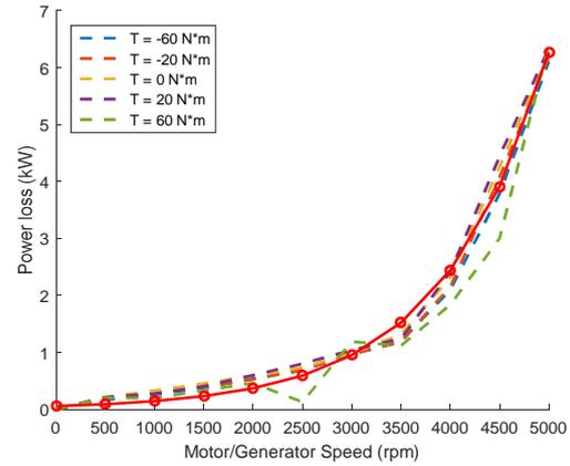
**Figure 3. Approximation of the motor/generator power losses.**
