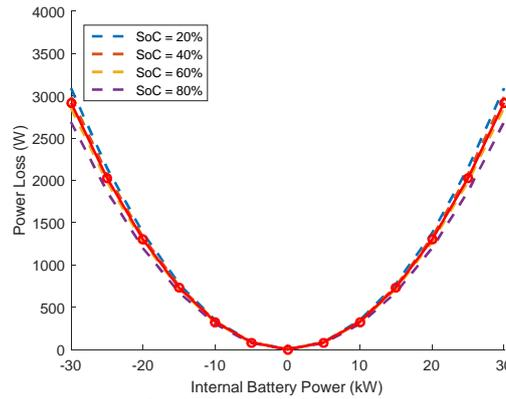
**Figure 4. Approximation of the battery power losses.**
