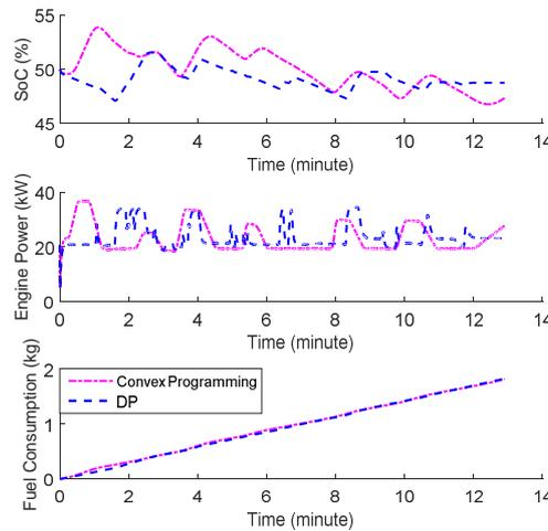
**Figure 8. Comparison of convex optimization and DP in test case 2.**
