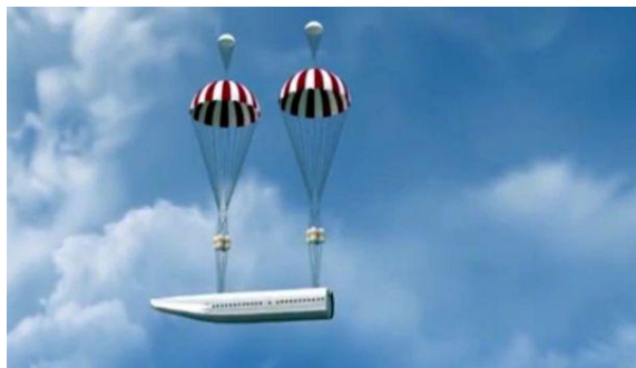
Figure 3: Braking of passengers' cabin falling with twin parachutes
