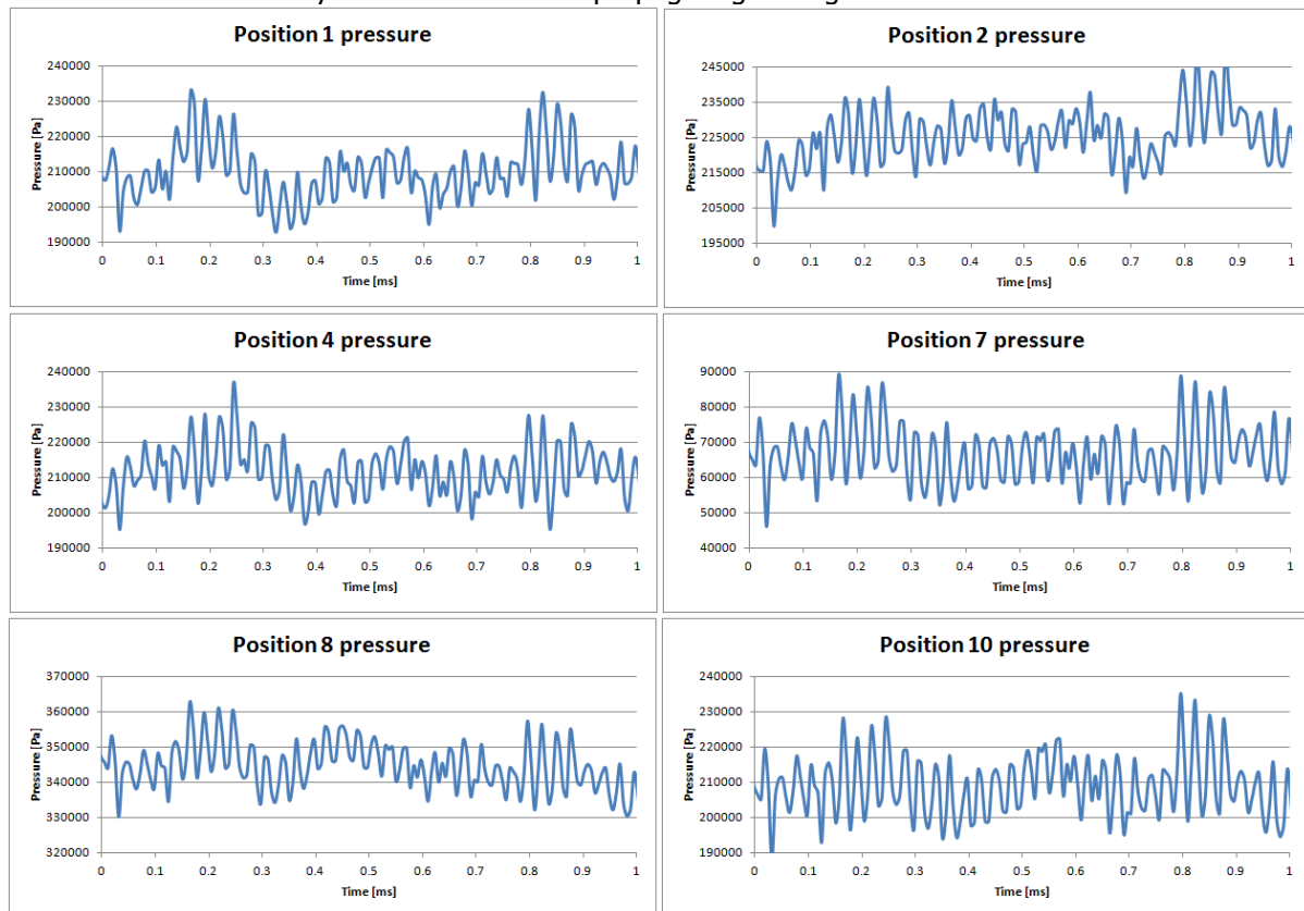
Figure 6: Pressure signal for baseline configuration under decreased inlet pressure
