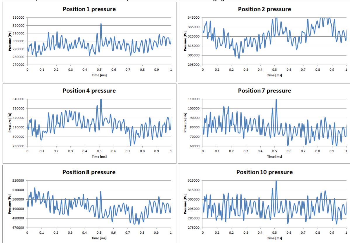
Figure 7: Pressure signal for baseline configuration under increased inlet pressure
