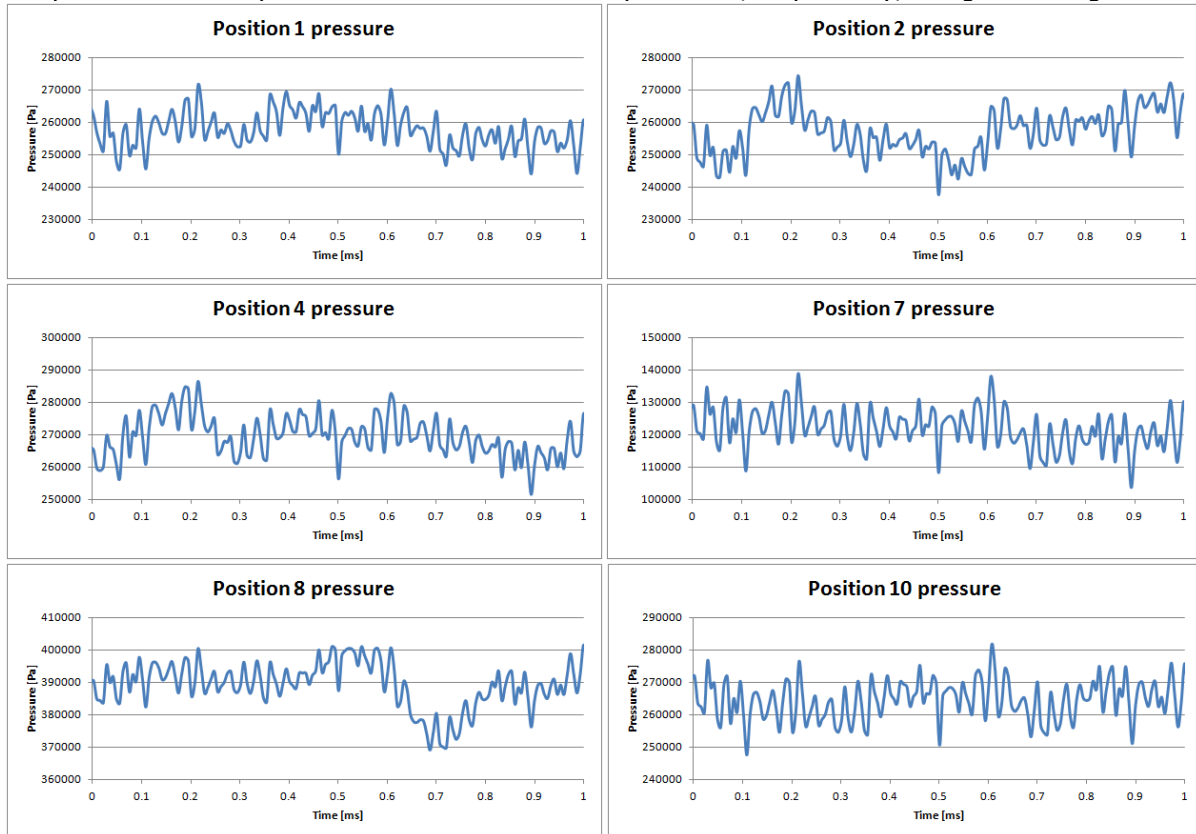
Figure 9: Pressure signal for the configuration with decreased critical section
