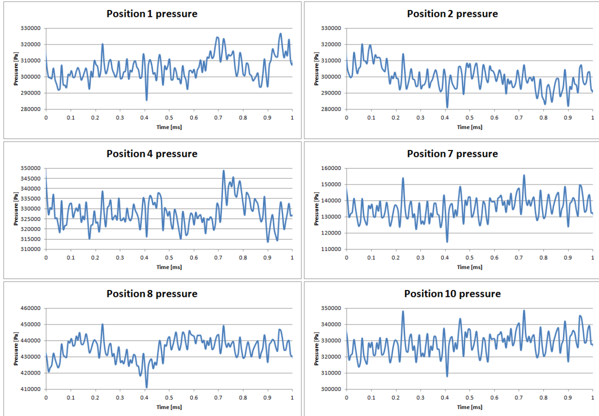
Figure 13: Pressure signal for the configuration with increased jet angle
