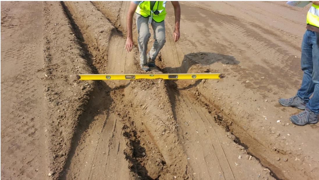
**Figure 7: 15 Deg oriented ruts profile distortion**
