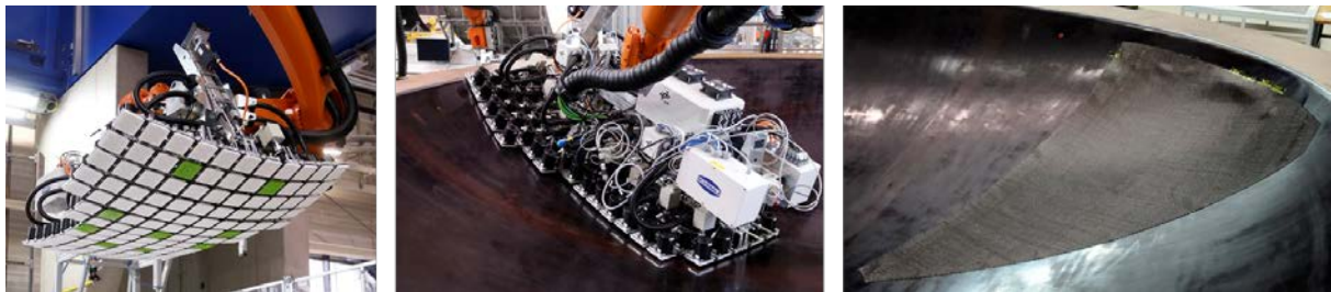
Figure 5: Draping by a kinematic gripper
