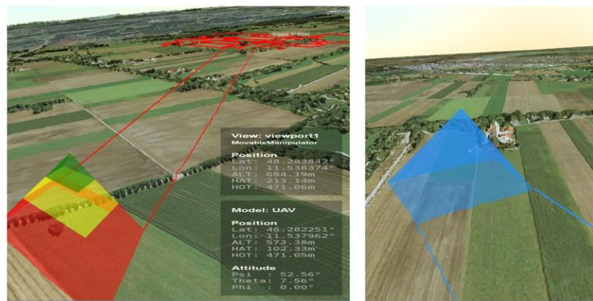
Figure 4: Color representation of the sensor's FOV and trail on the ground
