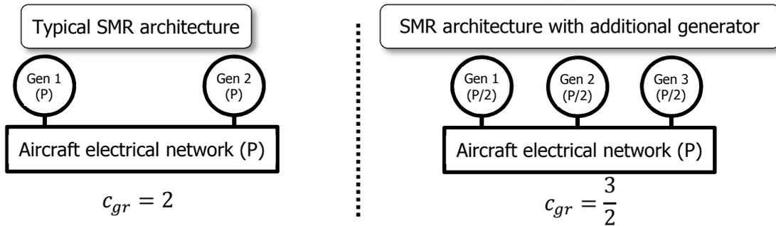
**Figure 8: Source sharing redundancy**
