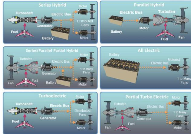
**Figure 4: Hybrid-electric propulsion architecture classifications [22]**
