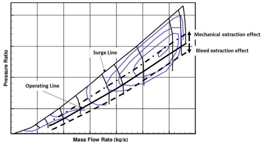
**Figure 3: Off-takes effect on HPC steady-state working line**
