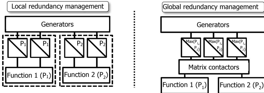
**Figure 9: Local and global electrical architecture view**
