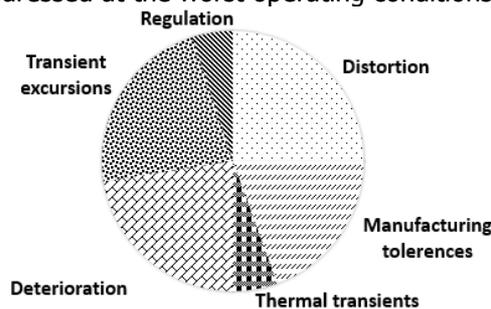
Figure 2: Typical turbofan HPC surge margin composition
