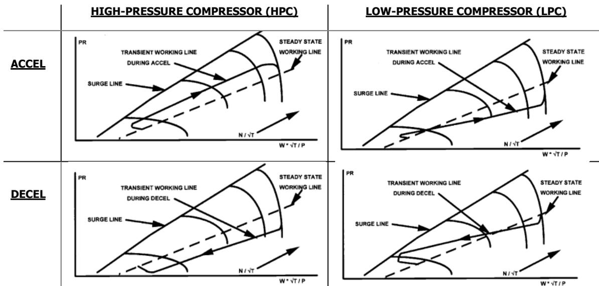
Figure 1: Typical transient working lines for gas turbine compressors [7]
