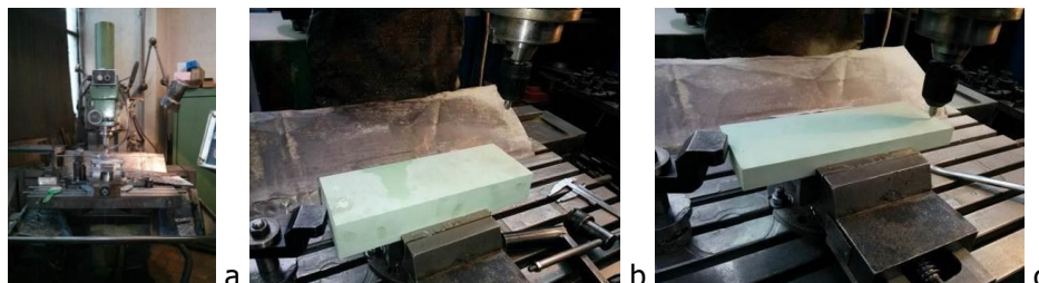
Figure 5. Manufacturing of the Necuron 702 mold components
