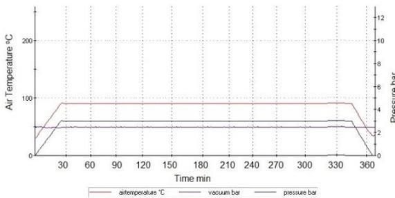
**Figure 15. Graphic representation of the curing cycle**
