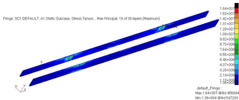
Figure 8. Maximum stress on the 4500 mm length spars
