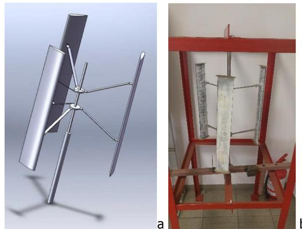
**Figure 10. (a) The CAD model of the VAWT with 4500 mm long blades; (b) Scaled (1:9) VAWT mounted on a metallic support**
