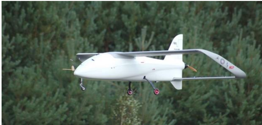
Figure 9: Aircraft in boxwing configuration built in the MOSUPS project.
