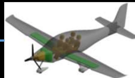
Cirrus SR-22 with Retrofit Electric Propulsion 200 nm range + reserves 11,300 lb
