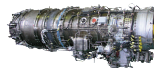
AI-222 versions with afterburner
