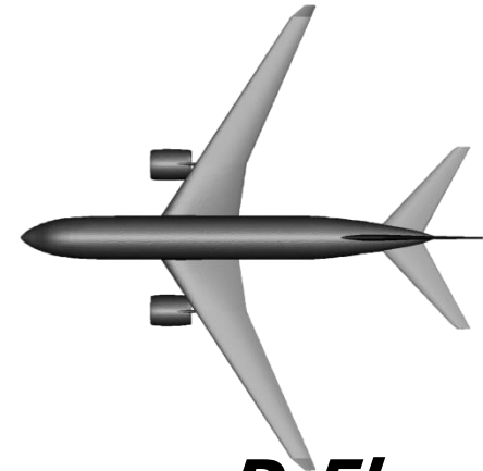
D-5k Direct flight variant 5000nm range
