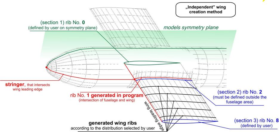
Airfoils are defined in separate files – four different formats are accepted (xfoil, koo, prf2, prf4)
