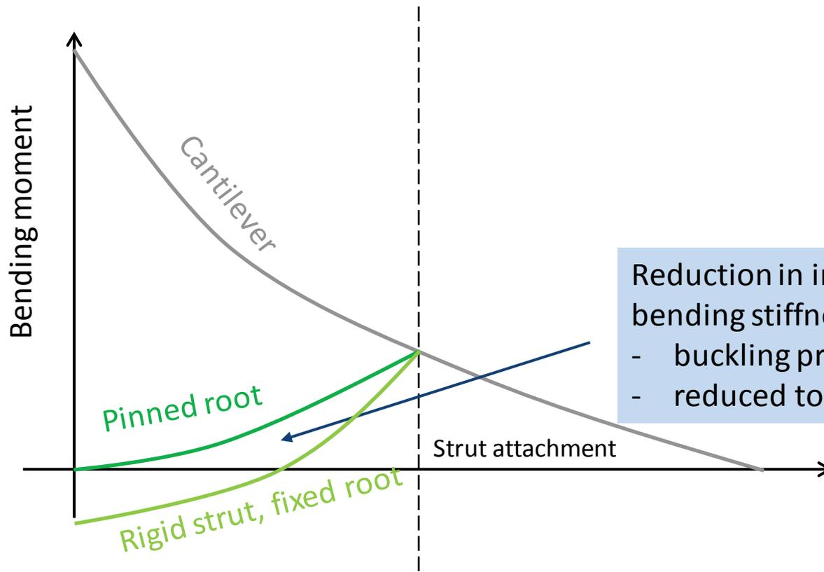
Reduction in inboard bending stiffness undesired
