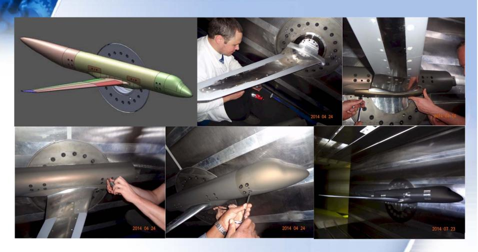
Assembling of the model for WT testing at CSIR
