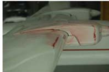
Flow visualization: laminar separation bubbles and transition strips
