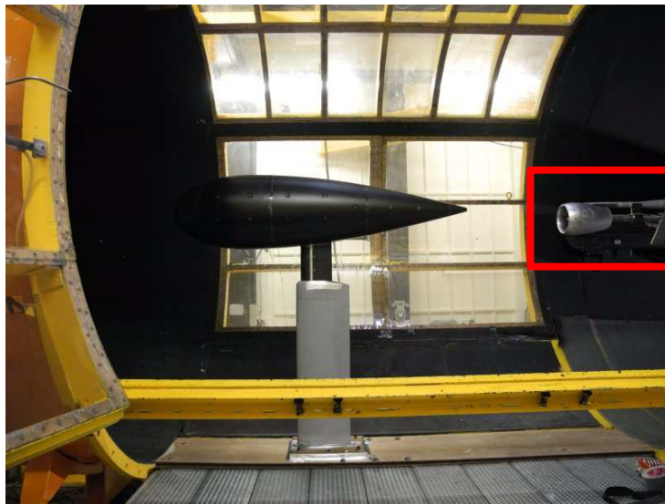
RAPRO2 test in ONERA L1 WT (Mach 0.2)
