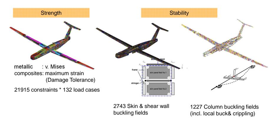
2.892.780 strength constraints 598.278 buckling constraints
